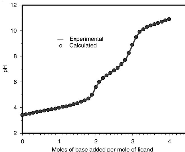
Fig. 3. Potentiometric titration curves for Cu(II)-ALA-Gly-Gly system at 25 °C and 0.10 mol L<sup>-1</sup> ionic strength
