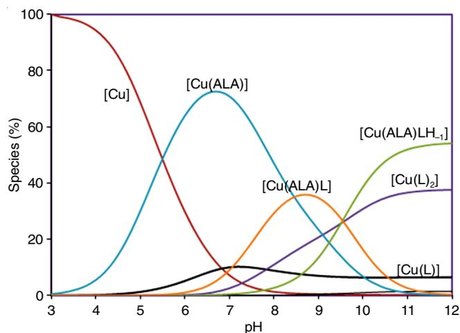
Fig. 4. Distribution curves as a function of pH calculated for  $\text{Cu}(\text{II})$ -ALA-Gly-Gly system at 25 °C and 0.10 mol L<sup>-1</sup> ionic strength of NaCl
