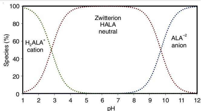
Fig. 1. Distribution curves as a function of pH calculated for ALA system at 25.0 °C and I = 0.10 mol L<sup>-1</sup> NaCl
