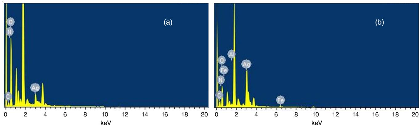
Fig. 7. The EDX spectrum of pure silver nanowire (a); and Ag@PCz nanocomposite (b)
