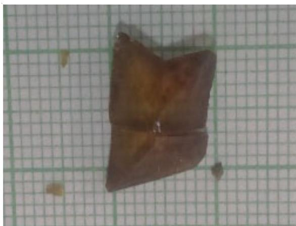
Fig. 1. Photograph of the grown MNBA crystal
