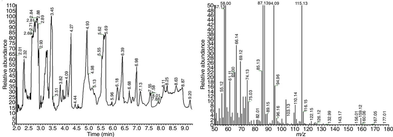
Fig. 1. Spectrogram of coconut shell LVM at pyrolysis temperature 600 °C
