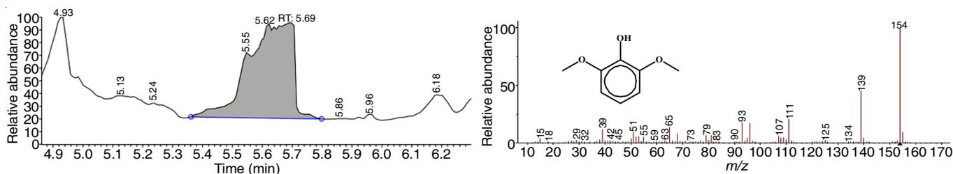
Fig. 6. Spectrogram 2,6-dimethoxy phenol compound of coconut shell LVM at pyrolysis temperature 600 °C
