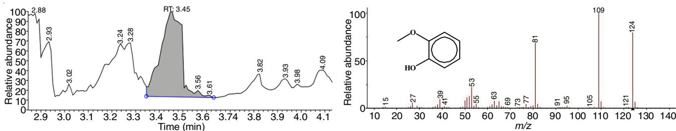
Fig. 4. Spectrogram 2,6-dimethoxy phenol compound of coconut shell LVM at pyrolysis temperature 600 °C
