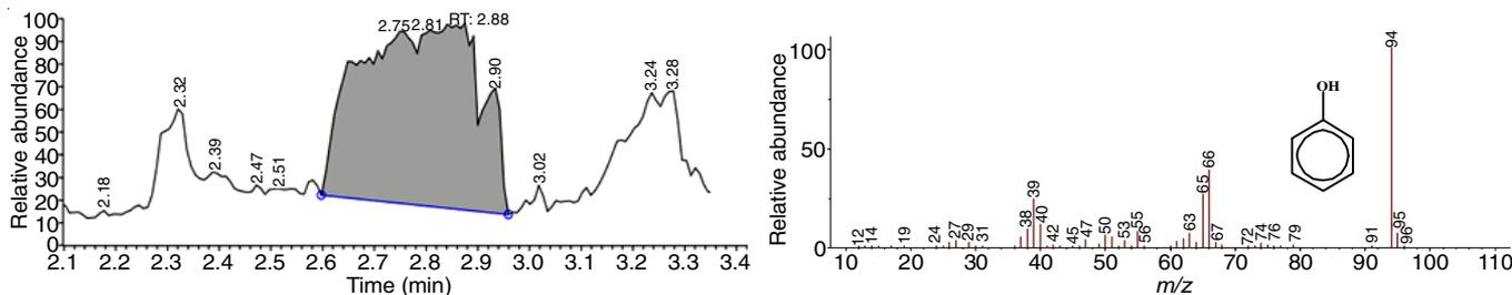
Fig. 2. Spectrogram phenol compound of coconut shell LVM at pyrolysis temperature 600 °C
