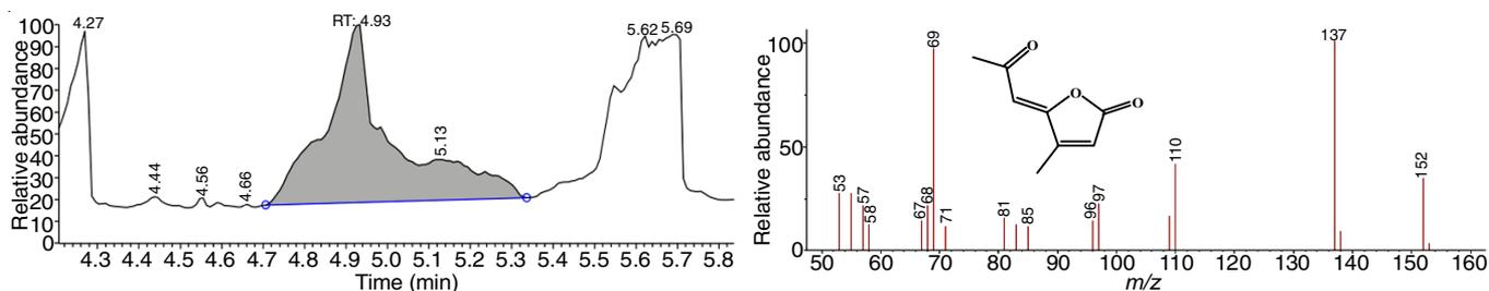
Fig. 5. Spectrogram (Z)-4-methyl-5-(2-oxopropylidene)-5H-furan-2-one compound of coconut shell LVM at pyrolysis temperature 600 °C
