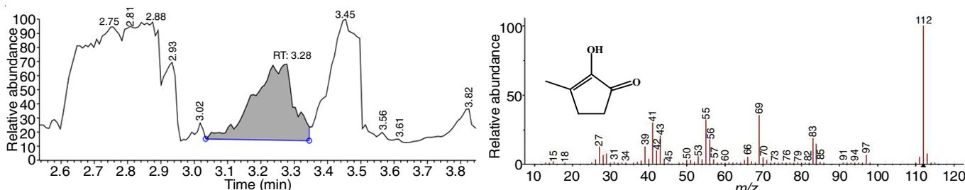
Fig. 3. Spectrogram 2-hydroxy-3-methyl 2-cyclopenten-1-one compound of coconut shell LVM at pyrolysis temperature 600 °C
