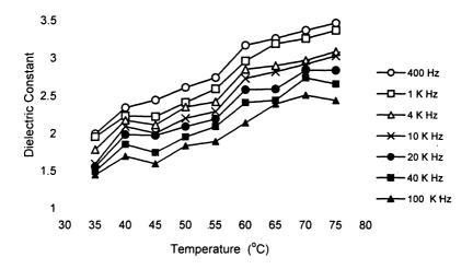
Fig. 1 Dependence of temperature on dielectric constant at different frequencies for red mud filled polymethyl methacrylate samples
