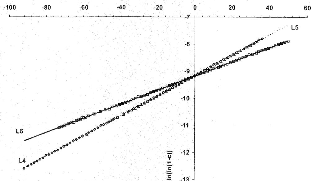
Fig. 4. Linearization curves of the first decomposition steps of Horowitz-Metzger methods for  $L^4$ ,  $L^5$  and  $L^6$
