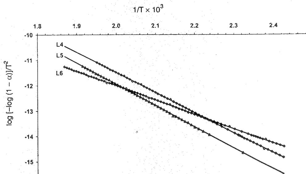
Fig. 3. Linearization curves of the first decomposition steps of Coats-Redfern methods for L<sup>4</sup>, L<sup>5</sup> and L<sup>6</sup>
