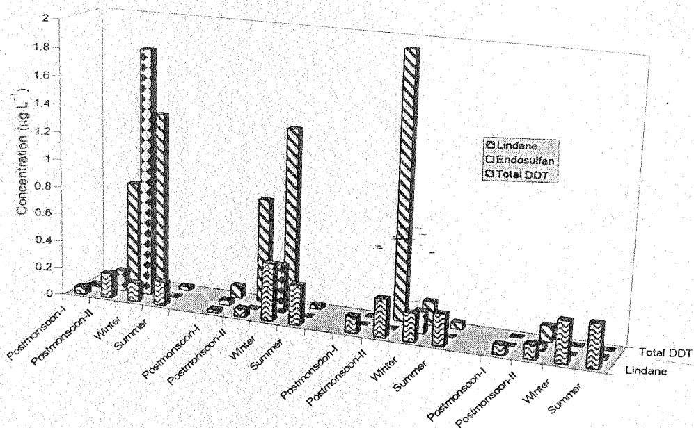
Fig. 4. Pesticide Levels in raw water at Mumbai (1995–96) (WHO guideline values for lindane 2 \mu\text{g L}^{-1} and DDT 1 \mu\text{g L}^{-1} )
