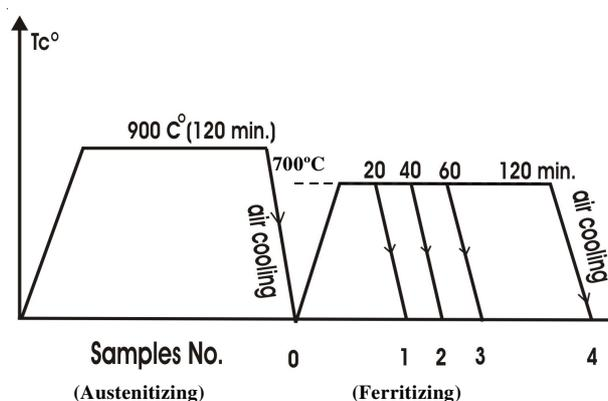
Fig. 1. Scheme of heat treatment of Ductil iron samples
