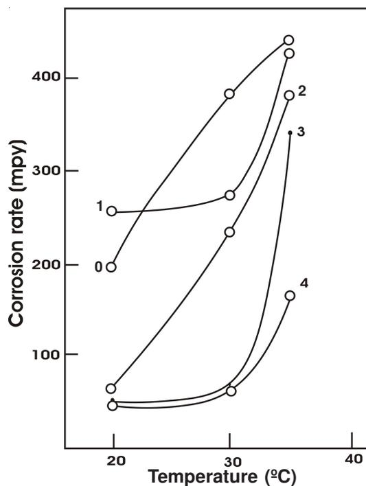
Fig. 4. Values of corrosion rate at different temperatures 20, 30, 35°C for samples no. 0, 1, 2, 3 and 4, respectively with increasing of ferritizing time
