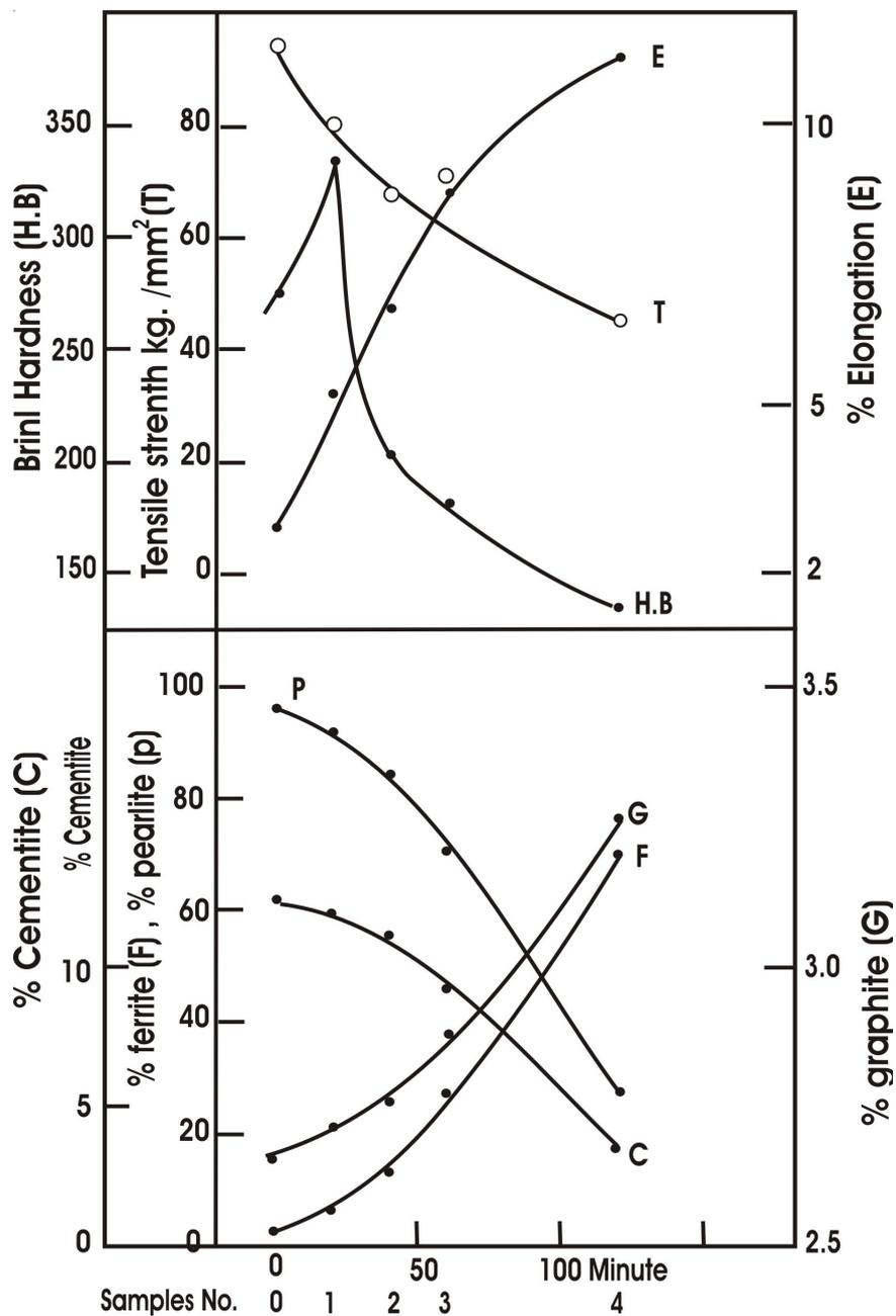
Fig. 2. Values of chemical and structure composition of ductile. Cast iron at different ferritizing times and corresponding physical (mechanical) properties
