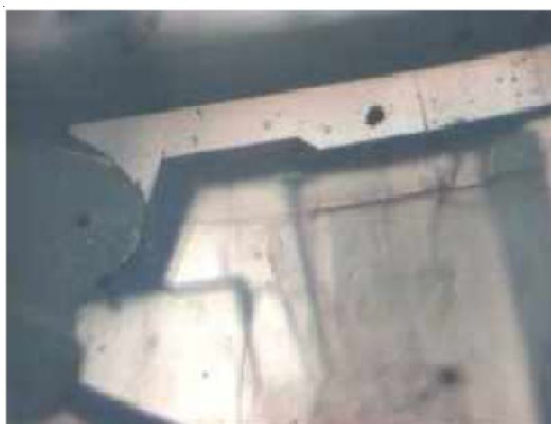
Fig. 5. Etch pits of CHP crystal (HCl of 1 N, 5 min etching time) at room temperature
