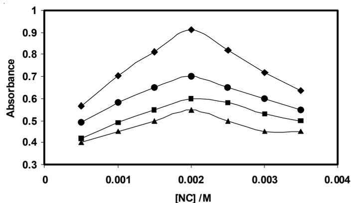
Fig. 1. Effect of concentration of neocuproine on the reaction of  $0.30 \mu\text{g mL}^{-1}$  of hydrazine (■),  $0.90 \mu\text{g mL}^{-1}$  of PHZ (▲),  $4.5 \mu\text{g mL}^{-1}$  of AHZ (●) and mixture of them (◆), Conditions:  $4 \times 10^{-3}$  M Cu(II), pH 6.0,  $25^\circ\text{C}$
