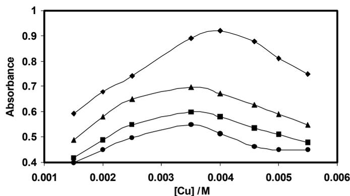
Fig. 2. Effect of concentration of Cu(II) on the reaction of  $0.30 \mu\text{g mL}^{-1}$  of HZ (■),  $0.90 \mu\text{g mL}^{-1}$  of PHZ (▲),  $4.5 \mu\text{g mL}^{-1}$  of AHZ (●) and mixture of them (◆). Conditions:  $2 \times 10^{-3}$  M neocuproine, pH 6.0,  $25^\circ\text{C}$
