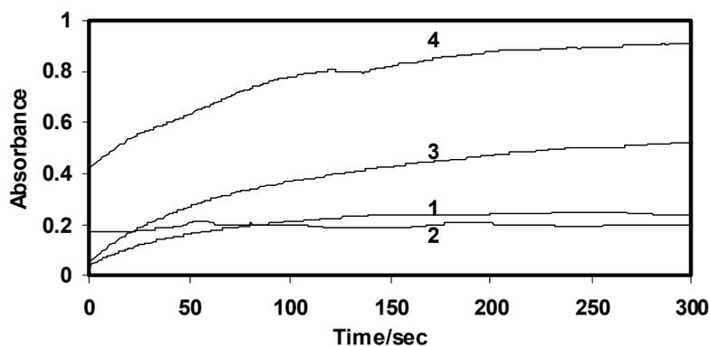
Fig. 4. Absorbance changes of Cu(II)/neocuproine complex vs. time in the reaction with: (1)  $0.30 \mu\text{g mL}^{-1}$  of HZ, (2)  $0.90 \mu\text{g mL}^{-1}$  of PHZ and (3)  $4.5 \mu\text{g mL}^{-1}$  of AHZ and mixture of them (4). Conditions:  $2.0 \times 10^{-3}$  M neocuproine,  $4.0 \times 10^{-3}$  M Cu(II), pH 6.0, 25 °C
