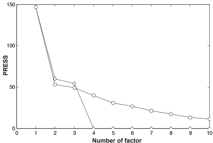
Fig. 5. Plot of PRESS against the number of factors for mixture of hydrazine, phenyl hydrazine and acetyl hydrazine for PLS (○) and PCR (◇) methods
