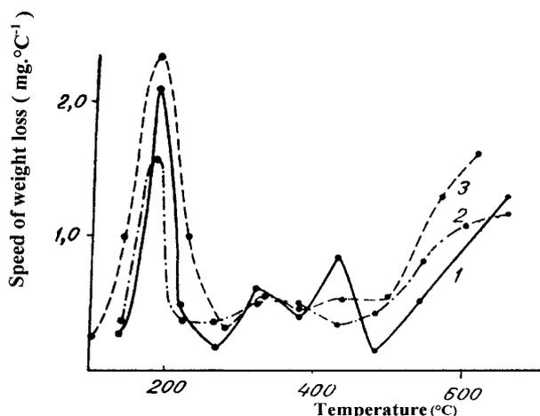
Fig. 1. Curves of the speed variation of the weight loss in function with the temperature of the poly-N-(4-vinylphenyl) alkyl dithiocarbamates
