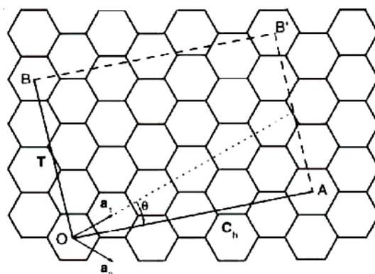
Fig. 1. Graphen sheet and chiral vector of carbon nanotubes
