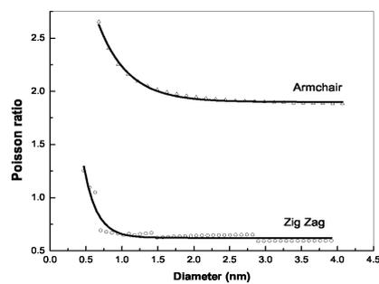
Fig. 5. Variation of Poisson ratio with nanotube diameter under Morse potential
