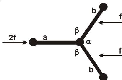
Fig. 2. Unit structure of an armchair nanotube
