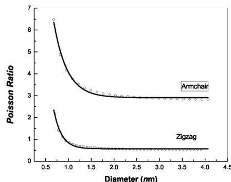
Fig. 7. Variation of Poisson ratio with nanotube diameter under harmonic potential
