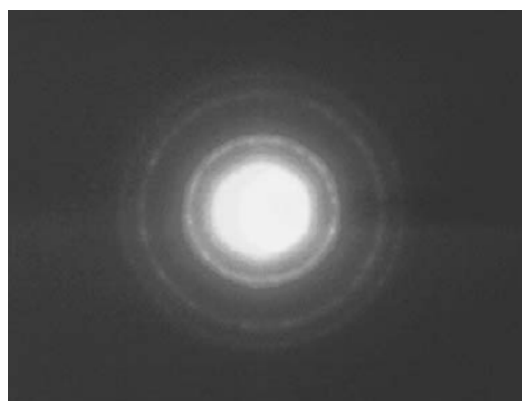
Fig. 2. Electron diffraction pattern of cubic diamond
