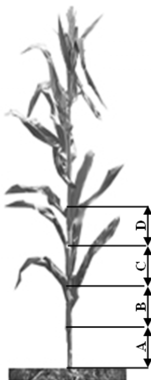
Fig. 1. Regions of the silage corn stalk at which measurements were made (A: 0-10 cm, B:10-20 cm, C:20-30 cm, D: 30-40 cm)
