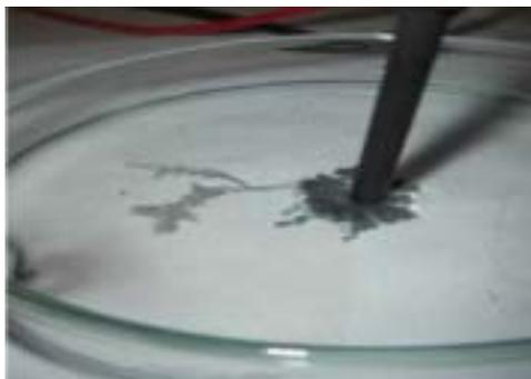
Fig. 2b. Zinc aggregate pattern at 3M conc. of zinc sulfate solution. Growth started within 1 min and got completed up to 15 min
