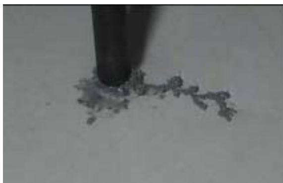
Fig. 6. Zinc aggregate pattern by using zinc chloride as an electrolyte. Growth started after few minutes and got completed up to 20 min
