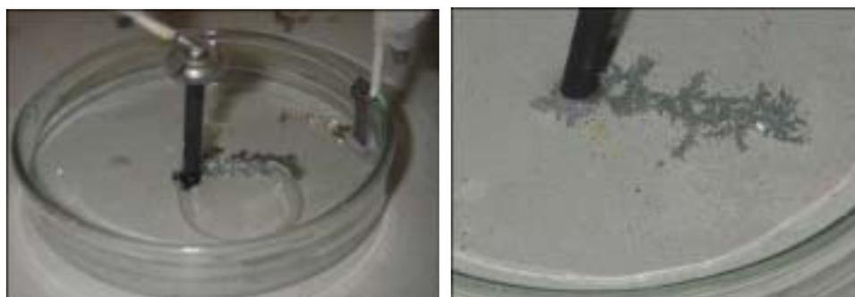
Fig. 5a. Zinc aggregate pattern by using chloroform solvent. Growth started immediately and got completed after 60 s
