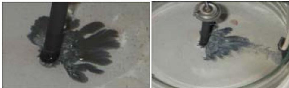
Fig. 4a. Zinc aggregate pattern at 8 volt potential. Growth started immediately and got completed within 30-60 s
