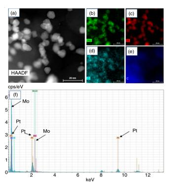
Fig. 3. (a) HR-TEM images of Pt-Mo (1:1)/Vulcan XC-72. Elemental mapping of (b) Mo, (c) Pt, (d) O and (e) C. (f) EDX analysis of Pt-Mo (1:1)/Vulcan XC-72 showing the presence of Mo and Pt
