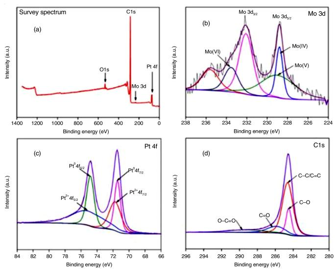
Fig. 2. XPS spectra of Pt-Mo (1:1)/Vulcan XC-72. (a) The survey spectrum, (b) Mo 3d, (c) Pt 4f, and (d) C 1s
