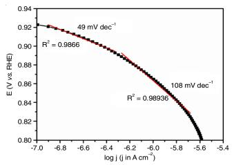
Tafel slope by plotting applied potential versus log of current density Fig. 6.
