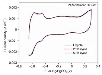
Fig. 4. Cyclic voltammogram of Pt-Mo (1:1)/Vulcan XC-72 at a scan rate of 50 mV  $\rm s^{\text{-}1}$
