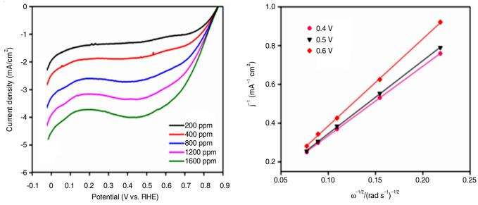
Fig. 5. (a) RDE measurements of Pt-Mo (1:1)/Vulcan XC-72 catalyst in O2 saturated 0.5M H2SO4 at a scan rate of 5 mV s<sup>-1</sup> and at different rotation speed (200, 400, 800, 1200 and 1600 rpm); (b) Koutechy-Levich plots (j<sup>-1</sup> versus ω<sup>-0.5</sup>) from RDE measurements of Pt-Mo (1:1)/C
