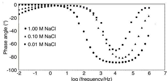
Fig. 5. Bode phase diagrams of BLM formed on electrochemically activated GCE surface
