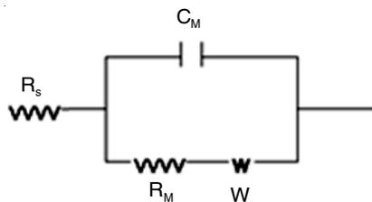
Fig. 3. Equivalent for BLM formed on electrochemically activated GCE surface
