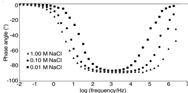
Fig. 7. Bode phase diagram of s-BLMs in the presence of 1 mM  $\text{Fe}(\text{CN})_6^{3-/4-}$  ions in NaCl bath solutions
