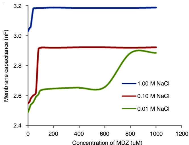
Fig. 8. Variation of membrane capacitance with drug dose in the presence of 1 mM  $\text{Fe}(\text{CN})_6^{3-/4-}$  ions
