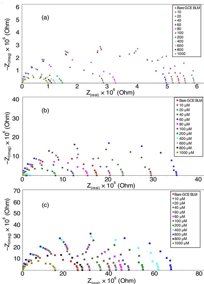
Fig. 6. Nyquist plots of bare and drug doped s-BLMs in 1.0 M, 0.1 M and 0.01 M NaCl bath solutions in the presence of 1 mM  $\text{Fe}(\text{CN})_6^{3-/4-}$  ions
