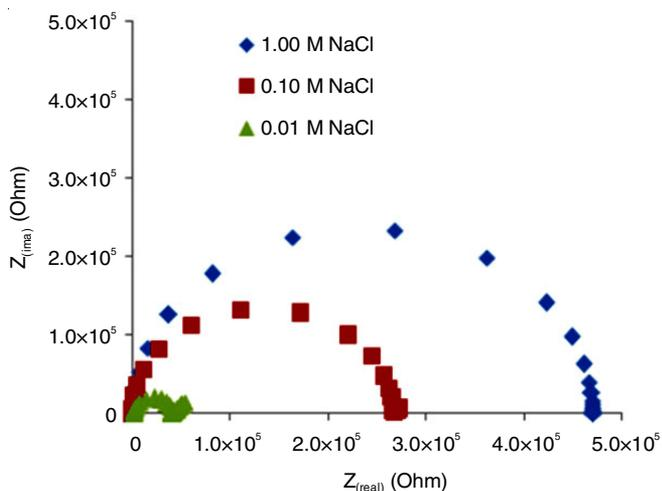
Fig. 2. Nyquist plots of BLM formed on electrochemically activated GCE surface in NaCl bath solutions
