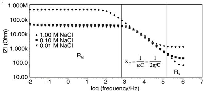
Fig. 4. Bode impedance plots of BLM formed on electrochemically activated GCE surface
