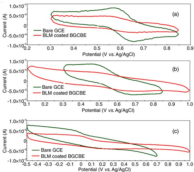
Fig. 9. Cyclic voltammetric response of bare and BLM coated GCEs in 1.0 M, 0.1 M and 0.01 M NaCl bath solutions respectively, containing 1:1 ratio of 1 mM of  $\text{Fe}(\text{CN})_6^{3-/4-}$  ions
