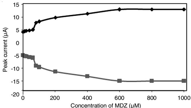
Fig. 11. Plot of redox peak currents ( $\mu\text{A}$ ) vs. concentration of MDZ ( $\mu\text{M}$ ) in the presence of 1:1 mM  $\text{Fe}(\text{CN})_6^{3-/4-}$  in 0.1 M NaCl bath solution at pH 7, scan rate  $100 \text{ mV s}^{-1}$
