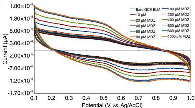
Fig. 10. Cyclic voltammetric response of  $\text{Fe}(\text{CN})_6^{3-/4-}$  ions at BLM coated GCE in 0.1 M NaCl bath solution at various concentration of MDZ
