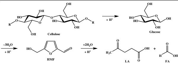
Scheme-I: Dehydration reaction mechanim of glucose to 5-HMF
