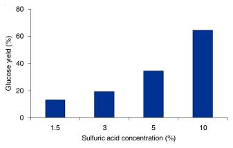
Fig 1. Effect of acid concentration on the hydrolysis of glucose
