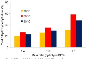
Fig. 5. Effect of DES on the Yield 5-HMF at varoius temperatures
