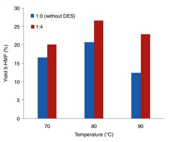
Fig. 3. Effect of deep euthetic solvent (DES) on the yield of 5-HMF
