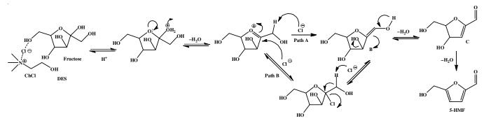
Fig. 4. Dehydration mechanism of glucose to 5-HMF in the presence of DES system (ChCl/citric acid::1:6) [Ref. 30]
