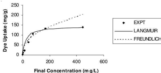
Fig. 5. Comparison of the experimental and predicted isotherms for reactive orange 16 on *Gracilaria verrucosa* (initial pH 4.0, temperature 30 °C,  $C_0 = 10$  mg/L, agitation rate 150 rpm).
