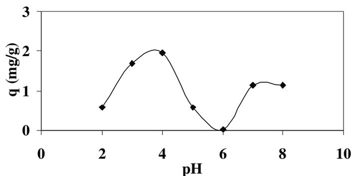
Fig. 1. Effect of initial pH on the equilibrium uptake capacity of *Gracilaria verrucosa* of reactive orange 16 (temperature 30 °C, agitation rate 150 rpm,  $C_0 = 10$  mg/L)
