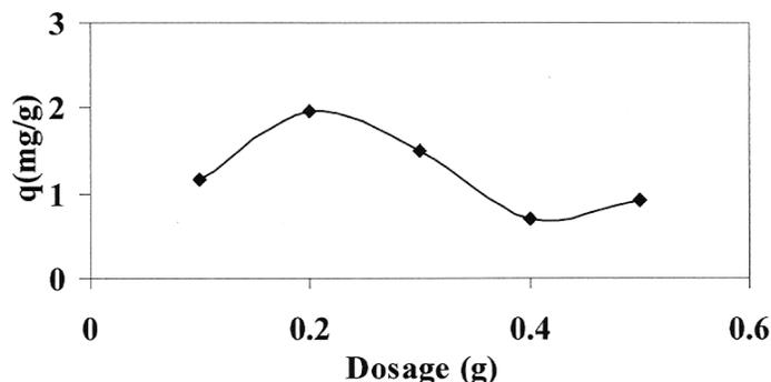
Fig. 3. Effect of dosage on the equilibrium uptake capacity of *Gracilaria verrucosa* of reactive orange 16 (initial pH 4.0, temperature 30 °C,  $C_0 = 10$  mg/L, agitation rate 150 rpm)
