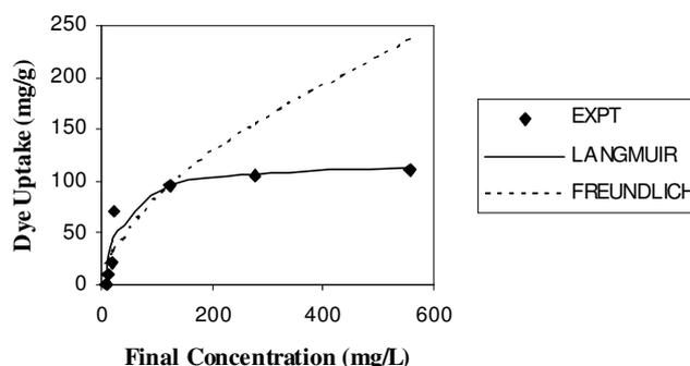
Fig. 6. Comparison of the experimental and predicted isotherms for reactive orange 16 on *Gracilaria verrucosa* (initial pH 4.0, temperature 30 °C,  $C_0 = 10$  mg/L, agitation rate 150 rpm)
