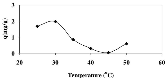
Fig. 2. Effect of temperature on the equilibrium uptake capacity of *Gracilaria verrucosa* of reactive orange 16 (initial pH 4.0, temperature 30 °C, Co = 10 mg/L, agitation rate 150 rpm)
