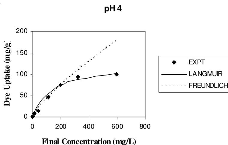
Fig. 4. Comparison of the experimental and predicted isotherms for reactive orange 16 on *Gracilaria verrucosa* (initial pH 4.0, temperature 30 °C,  $C_o = 10$  mg/L, agitation rate 150 rpm)
