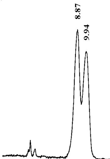
Fig. 6. Separation of the enantiomers of phthalylvaline. Wavelength 245 nm, flow rate 1 mL/min, volume injected 5  $\mu$ L. Column, Si-QN (250 mm  $\times$  6 mm, 12 mm). Mobile phase, methanol/acetic acid (99.5/0.5 v/v), 0.125mg sodium acetate
