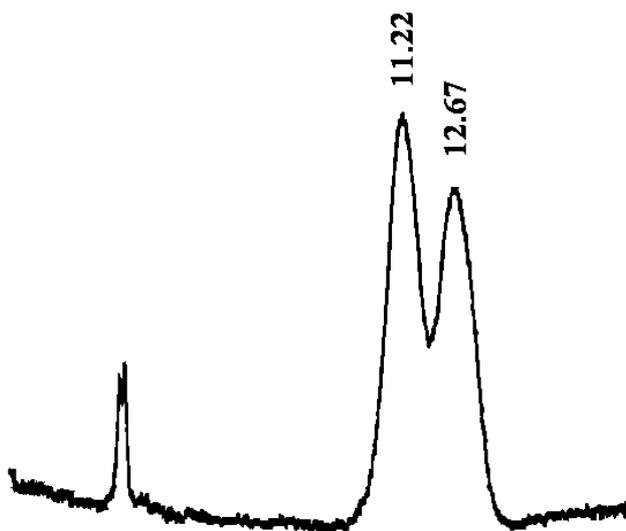
Fig. 4. Separation of the enantiomers of phthalylvaline. Wavelength 245 nm, flow rate 1 mL/min, volume injected 5  $\mu$ L. Column, Si-QN (250 mm  $\times$  6 mm, 12 mm). Mobile phase, methanol/acetic acid (99.5/0.5 v/v)
