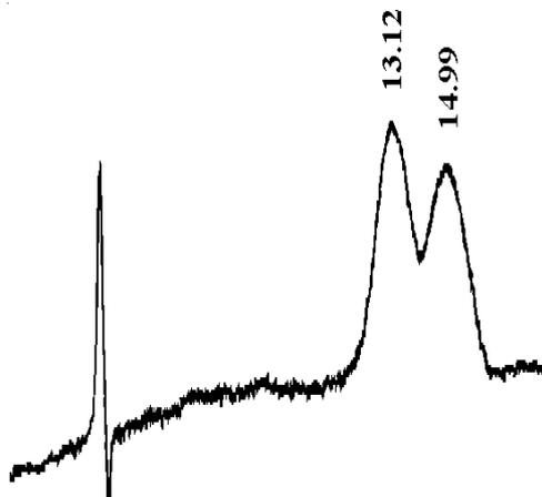
Fig. 5. Separation of the enantiomers of phthalylvaline. Wavelength 245 nm, flow rate 1 mL/min, volume injected 5  $\mu$ L. Column, Si-QN (250 mm  $\times$  6 mm, 12 mm). Mobile phase, Methanol/propanoic acid (99.5/0.5 v/v)
