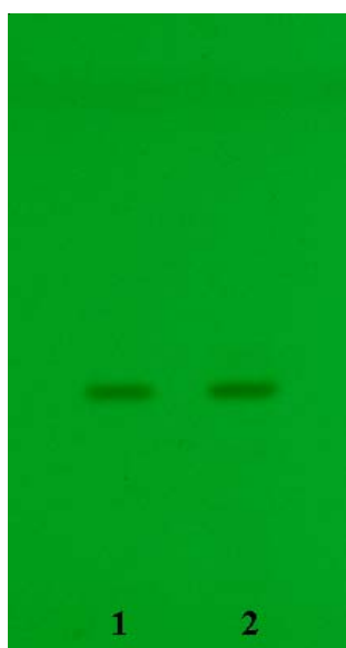
Fig. 3. Photograph of developed plate at 257 nm; Track 1) Sample ( Pueraria tuberosa DC.); 2) Standard (Puerarin)
