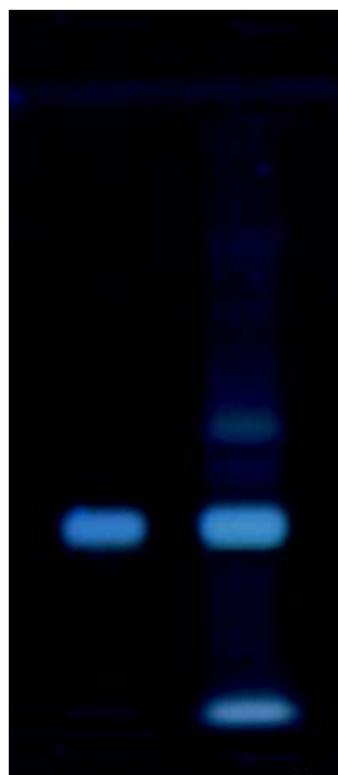
Fig. 4. Photograph of developed plate at 366 nm; Track 1) Standard ( \beta -sitosterol); 2) Sample ( Pueraria tuberosa DC.)
