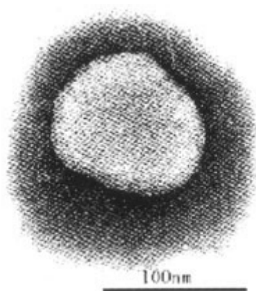
Fig. 3. TEM image of SiO 2 /polyurethane nanocomposite with the ratio of 2:10 by weight between tetraethoxy silane and polyurethane
