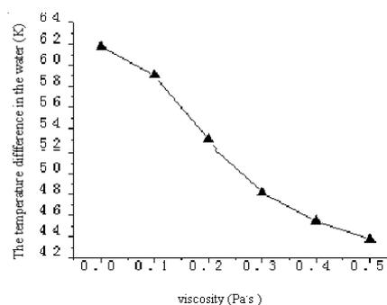
Fig. 9. The curve of difference in temperature at different viscosity without stir
