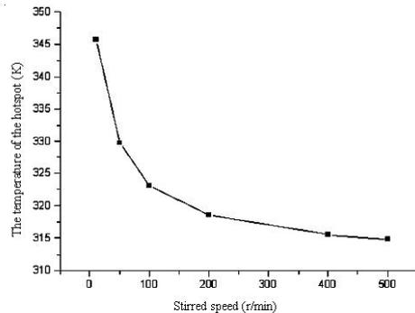
Fig. 4. The highest temperature curve at different stirred speed
