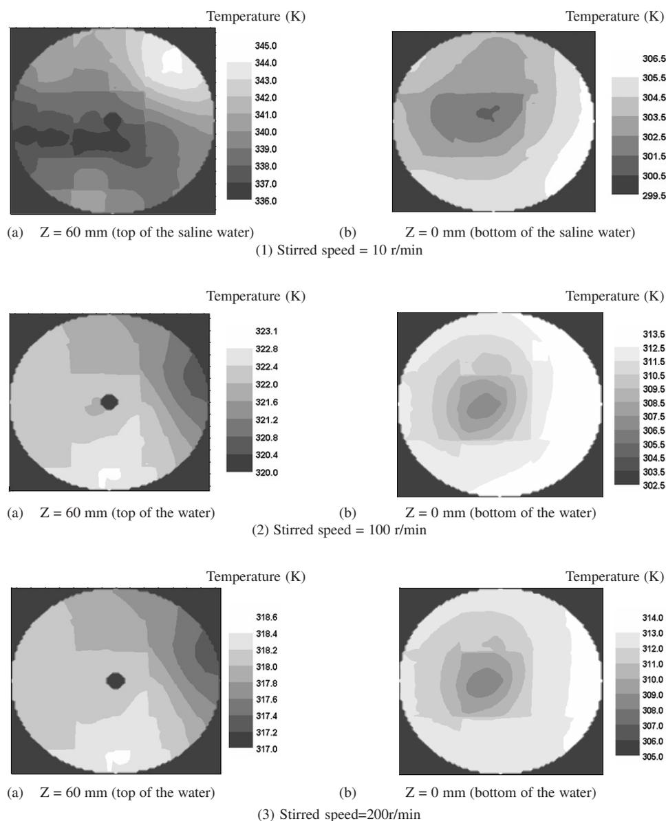
Fig. 3. Temperature distribution in the saline water after simulating 30 s different stirred speeds
