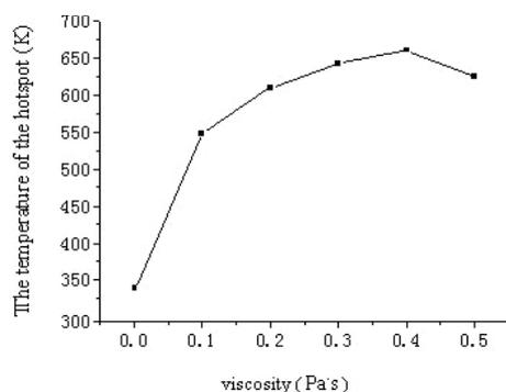
Fig. 8. The highest temperature curve at different viscosity without stir
