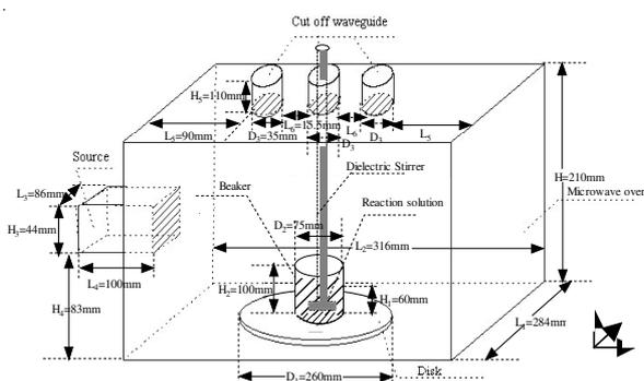
Fig. 2. The numerical simulation model
