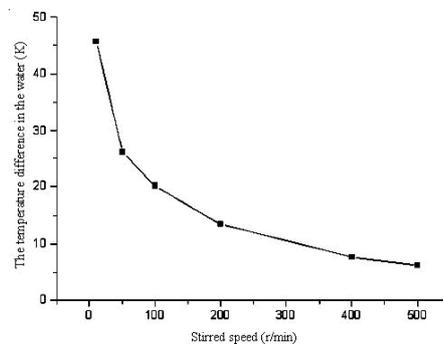
Fig. 5. The curve of difference in temperature at different stirred speed
