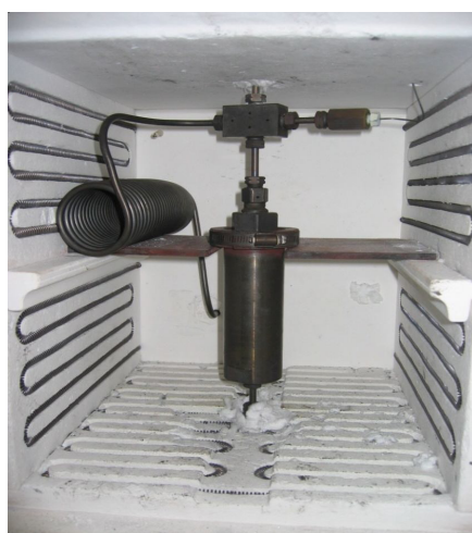
Fig. 3. Reactor/feeding assembly located inside the furnace
