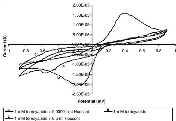
Fig. 3. Cyclic voltammogram (100 mV/s) of 1 mM ferricyanide alone and in the presence of Hoechst 33258
