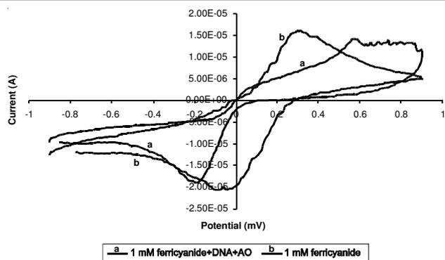
Fig. 2. Cyclic voltammogram (100 mV/s) of 1 mM ferricyanide alone and in the presence of ctDNA and acridine orange
