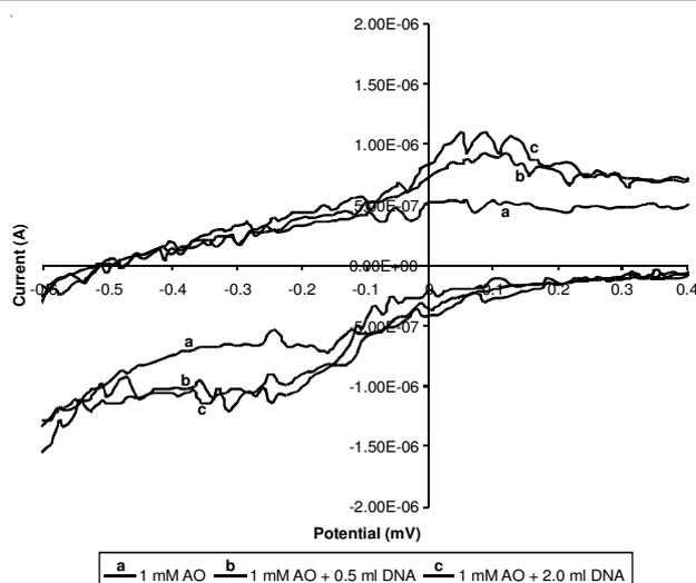
Fig. 9. Cyclic voltammogram (100 mV/s) of 1 mM acridine orange alone and with increasing amounts of ctDNA solution (400 ppm)
