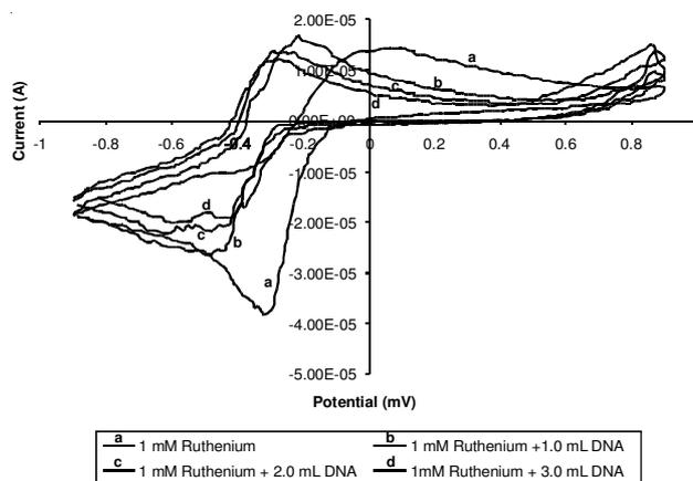
Fig. 5. Cyclic voltammogram (100 mV/s) of 1 mM ruthenium alone and in the presence of increasing amounts of ctDNA solution (400 ppm)
