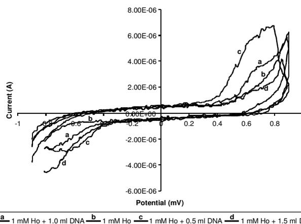
Fig. 8. Cyclic voltammogram (100 mV/s) of 1 mM Hoechst 33258 alone and with increasing amounts of ctDNA solution (400 ppm)
