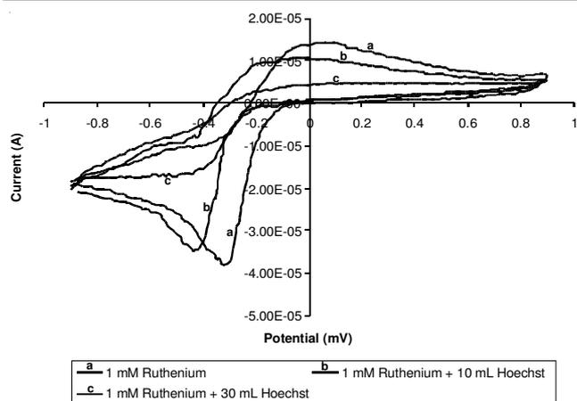
Fig. 6. Cyclic voltammogram (100 mV/s) of 1 mM ruthenium alone and in the presence of Hoechst 33258
