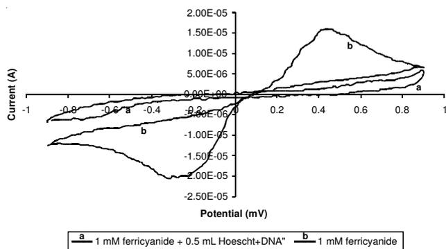
Fig. 4. Cyclic voltammogram (100 mV/s) of 1 mM ferricyanide alone and in the presence of Hoechst 33258 and ctDNA
