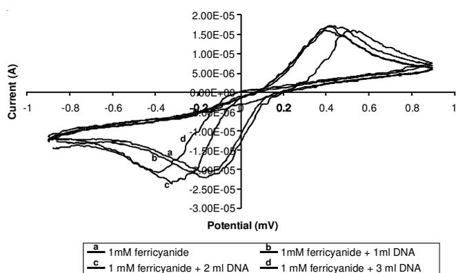
Fig. 1. Cyclic voltammogram (100 mV/s) of 1 mM ferricyanide alone and in the presence of increasing amounts of ctDNA solution (400 ppm) using a glassy carbon electrode in 0.1 M KCl
