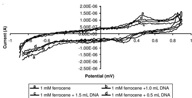
Fig. 7. Cyclic voltammogram (100 mV/s) of 1 mM ferrocene alone and with increasing amounts of ctDNA solution (400 ppm)
