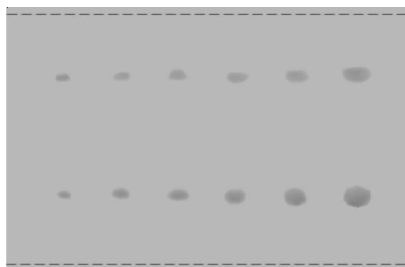
Fig. 6. TLC Plate of standard LOK and HCTZ for concentrations of each vitamin 1.0, 2.0, 4.0, 6.0, 8.0 and 10.0 \mu g/spot (mobile phase: phosphate buffer (10 mmol L^{-1} ; pH 3.2) and acetonitrile (60:40, v/v))
