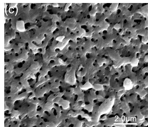
Fig. 1. Effect of dopants on morphology of thin TiO<sub>2</sub> film: (a) TiO<sub>2</sub>; (b) N-TiO<sub>2</sub>; (c) S-TiO<sub>2</sub>
