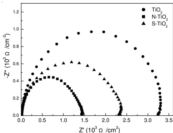
Fig. 2. Impedance spectra of cells assembled N-doped and S-doped  $\text{TiO}_2$  electrodes
