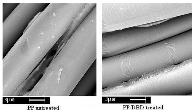
Fig. 4. SEM images of untreated and DBD treated polypropylene fabric
