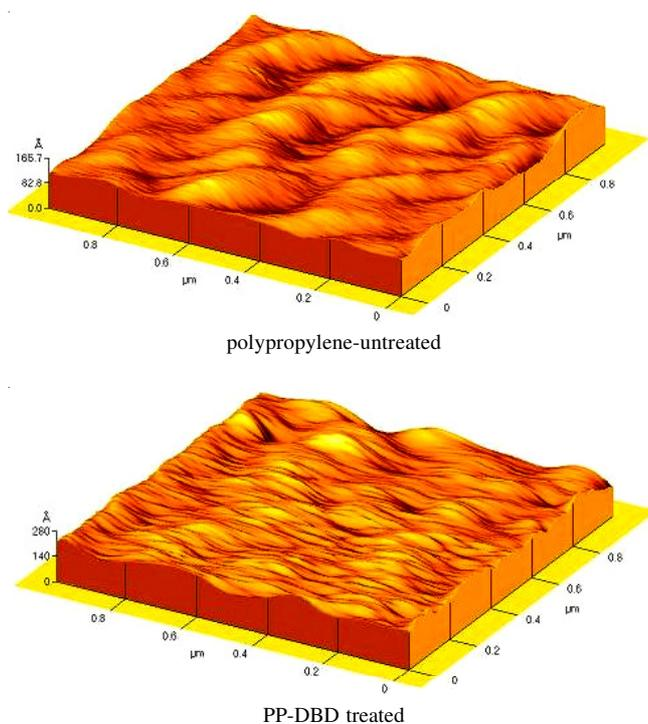
Fig. 3. Atomic force microscope images of untreated and DBD treated polypropylene foil
