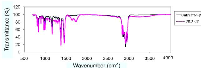
Fig. 2. FTIR spectra of untreated and DBD treated PP fabric
