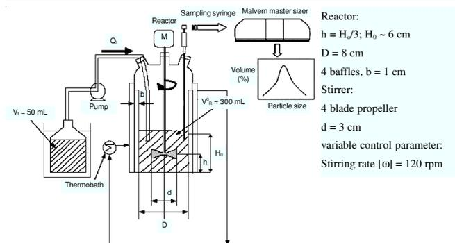
Fig. 1. Schematic diagram of single-feed semi-batch precipitation system
