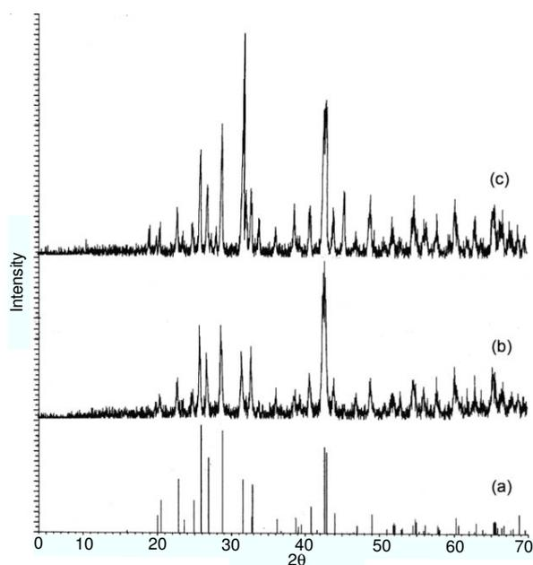
Fig. 2. XRD pattern of  $\text{BaSO}_4$  powders
