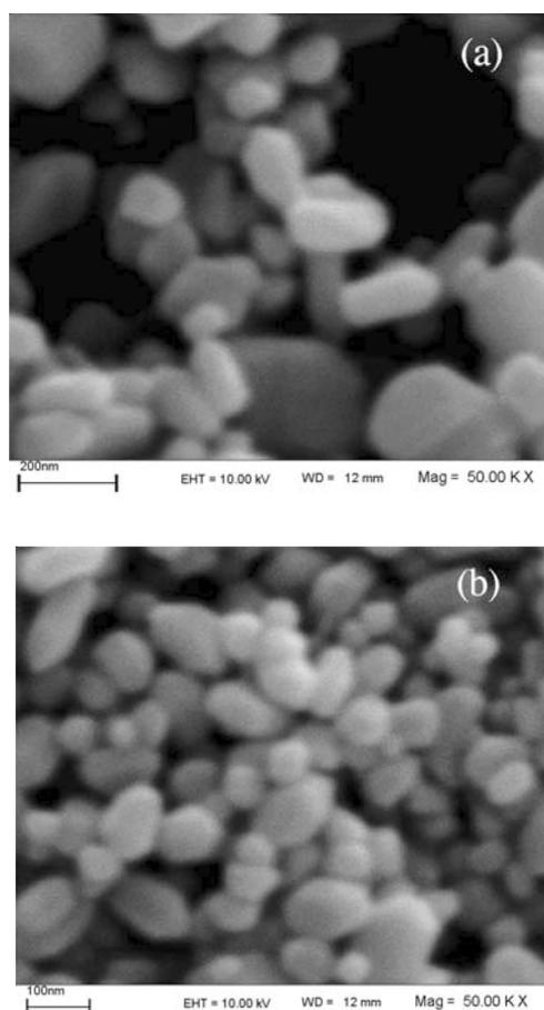
Fig. 3. SEM photography of  $\text{BaSO}_4$ : (a) from products in pure water and (b) from products obtained in the presence of ethanol
