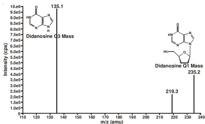
Fig. 2. Mass spectra of didanosine for parent and product masses
