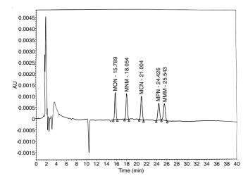
Fig. 1. Chromatogram of MON, MNM, MCN, MPN and MMM obtained with conditions optimized
