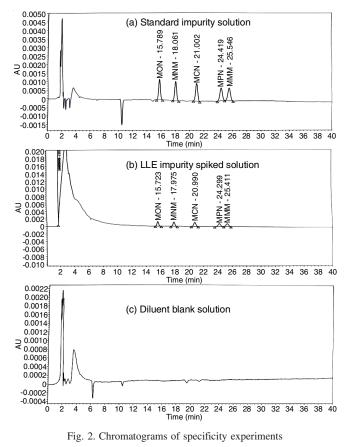
The diluent blank was infused and analyzed using proposed method. The chromatogram collected (Fig. 2c) did not display any peak at the MCN, MMM, MON, MPN and MNM retention times.
