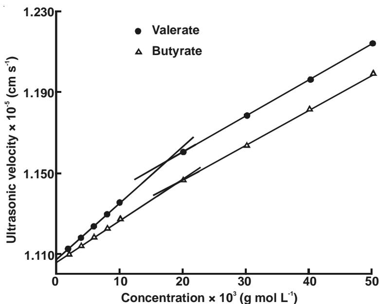
Fig. 1. Ultrasonic velocity vs. concentration of dysprosium soaps in methanol
