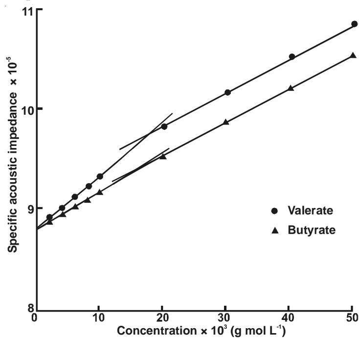
Fig.3 Specific acoustic impedance vs. concentration of dysprosium soaps in methanol
