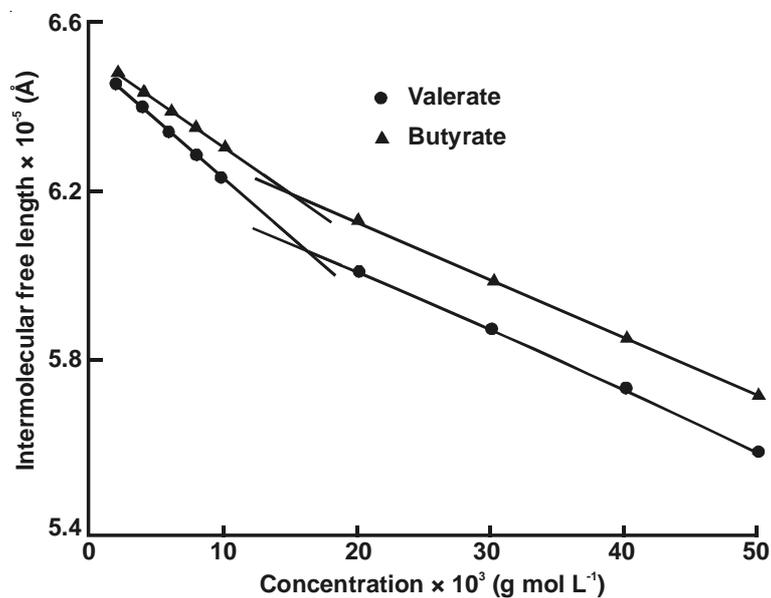
Fig.2 Intermolecular free length vs. concentration of dysprosium soaps in methanol
