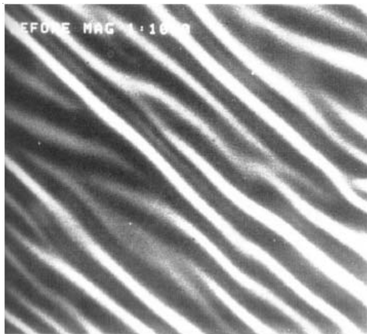
Fig. 7. Macroscopic appearance of the surface of azo crosslinked polyHEMA styrene (4:6) before incubation in the culture of E. faecalis
