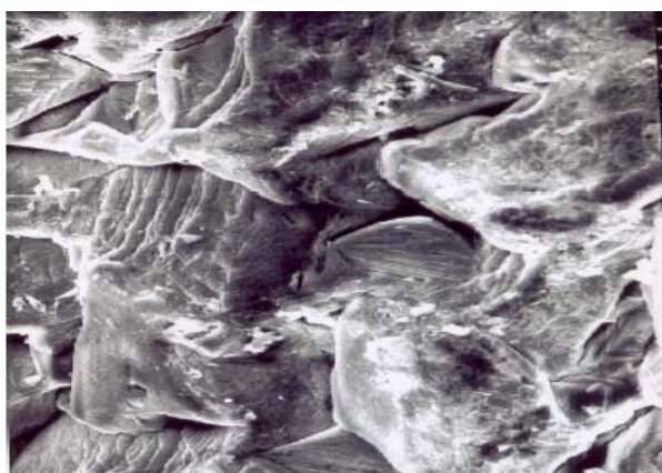
Fig. 7. Scanning electron microscopy of struvite crystals
