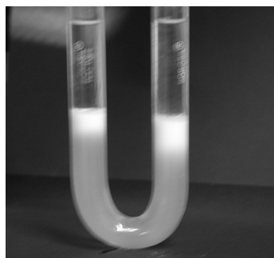
Fig. 2. SHP crystal growth in DDM-U tube
