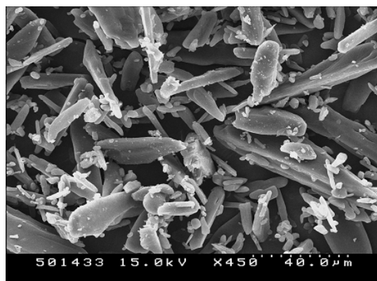
Fig. 3. SEM image of acetaminophen before ASES process
