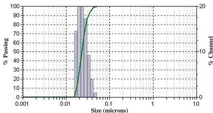
Fig. 2. Particle size analysis for  $\text{Fe}(\text{OH})_3$  nanofluid
