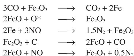
However, the results also indicate that the additive may be tried for NOx reduction in similar systems by using higher concentrations of Fe metal and more work is required in this direction.
