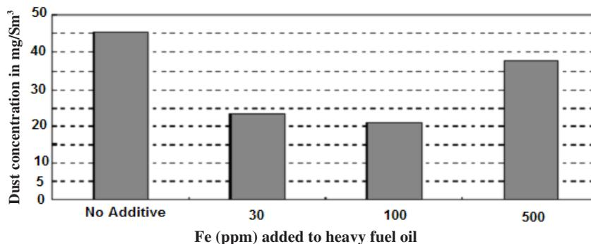
Fig. 3. Effect of Fe-nanofluid on particulate matter reduction
