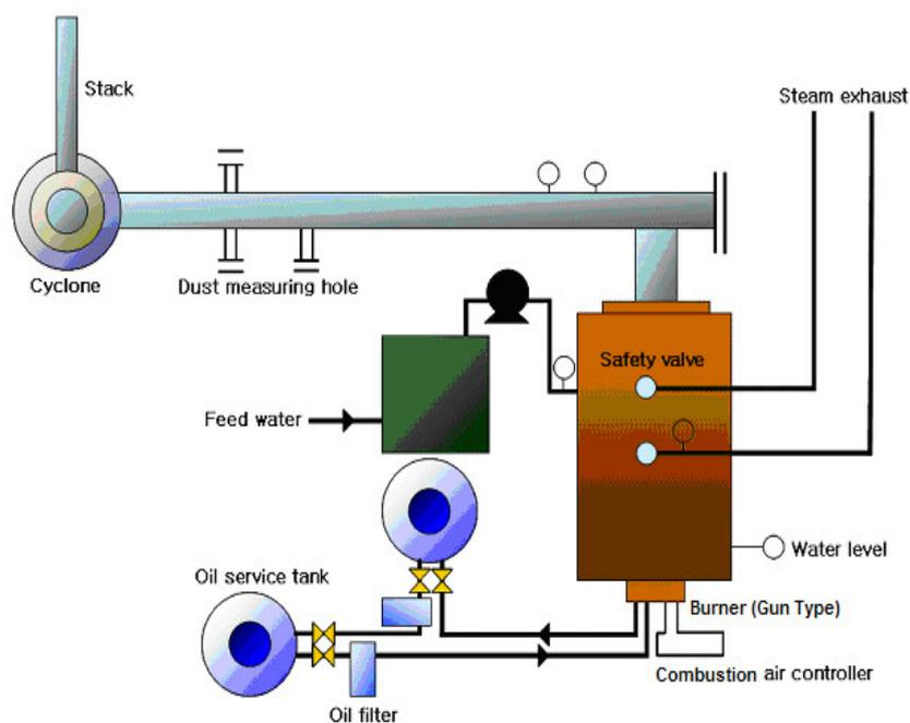
Fig. 1. Experimental setup of combustion boiler used for dust reduction
