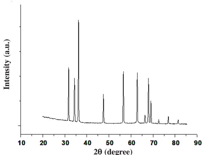
Fig. 2. XRD pattern of decomposition residue
