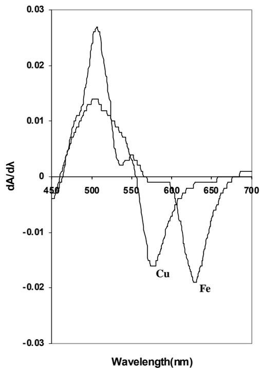
Fig. 4. First order derivative spectra of Cu(II)-PAN and Fe(III)-PAN complexes in AOT micellar solution. Conditions:  $2 \mu\text{g mL}^{-1}$  of Cu(II),  $2 \mu\text{g mL}^{-1}$  of Fe(III),  $0.006 \text{ mol L}^{-1}$  AOT,  $2 \times 10^{-4} \text{ mol L}^{-1}$  PAN and  $\text{pH} = 2.5$
