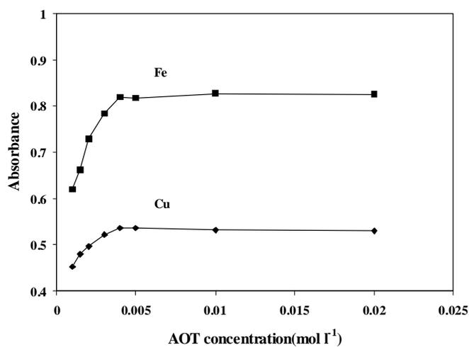
Fig. 5. Effect of AOT concentration on the absorbance (at  $\lambda_{\text{max}}$ ) of the Cu(II)-PAN and Fe(III)-PAN complexes. Conditions:  $2 \mu\text{g mL}^{-1}$  of Cu(II),  $2 \mu\text{g mL}^{-1}$  of Fe(III),  $2 \times 10^{-4} \text{ mol L}^{-1}$  PAN and  $\text{pH} = 2.5$
