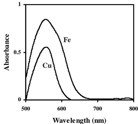
Fig. 2. Absorption spectra of Cu(II)-PAN and Fe(III)-PAN complexes in SDS micellar solution. Conditions:  $2 \mu\text{g mL}^{-1}$  of Cu(II),  $2 \mu\text{g mL}^{-1}$  of Fe(III),  $0.02 \text{ mol L}^{-1}$  SDS,  $2 \times 10^{-4} \text{ mol L}^{-1}$  PAN and pH = 2.5
