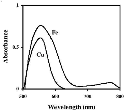
Fig. 1. Absorption spectra of Cu(II)-PAN and Fe(III)-PAN complexes in Triton-X-100 micellar solution. Conditions:  $2 \mu\text{g mL}^{-1}$  of Cu(II),  $2 \mu\text{g mL}^{-1}$  of Fe(III), 1.5 % (v/v) Triton-X-100,  $2 \times 10^{-4} \text{ mol L}^{-1}$  PAN and pH = 2.5
