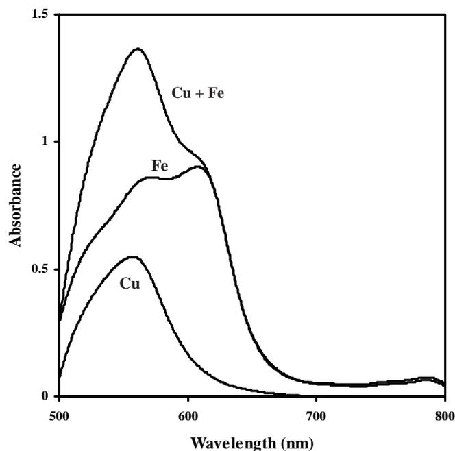
Fig. 3. Absorption spectra of Cu(II)-PAN, Fe(III)-PAN and mixture of Cu(II)-PAN + Fe(III)-PAN complexes in AOT micellar solution. Conditions:  $2 \mu\text{g mL}^{-1}$  of Cu(II),  $2 \mu\text{g mL}^{-1}$  of Fe(III),  $0.006 \text{ mol L}^{-1}$  AOT,  $2 \times 10^{-4} \text{ mol L}^{-1}$  PAN and pH = 2.5
