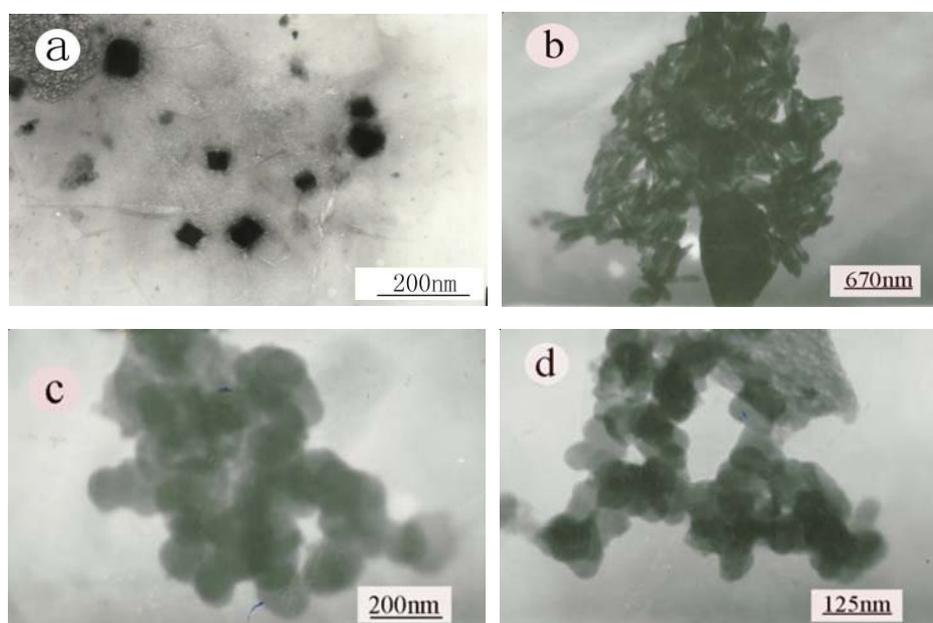
Fig. 1. Morphologies of  $\text{CaC}_2\text{O}_4$  crystals gained from different systems, (a-d) Microemulsions (I)–(V), respectively
