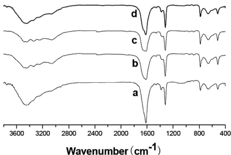
Fig. 2. FT-IR spectra of  $\text{CaC}_2\text{O}_4$  crystals grown in different systems, (a-d) Microemulsions (I)-(IV), respectively
