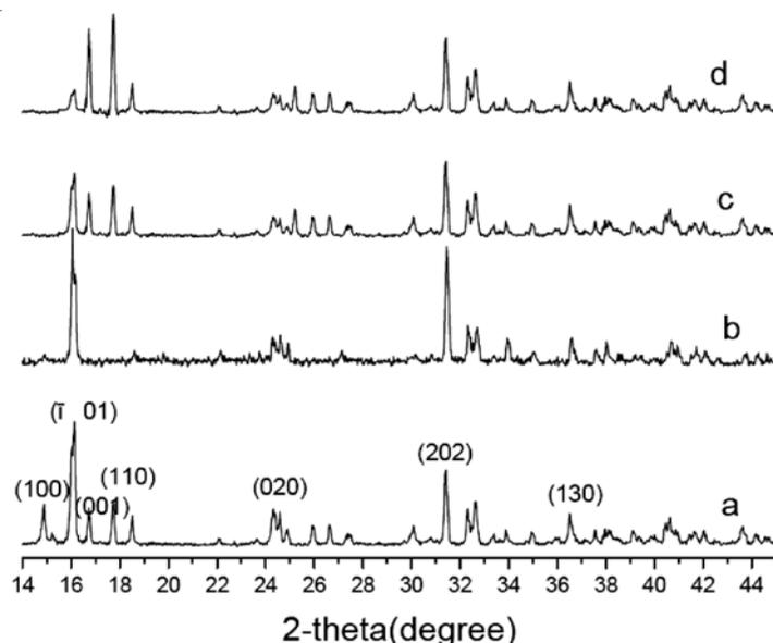
Fig. 3. XRD patterns of crystals produced in different systems, (a-d) Microemulsions (I)–(V), respectively
