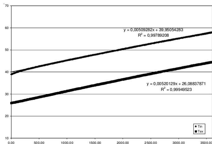
Fig. 11. Temperature *versus* time for P = 16.0 W
