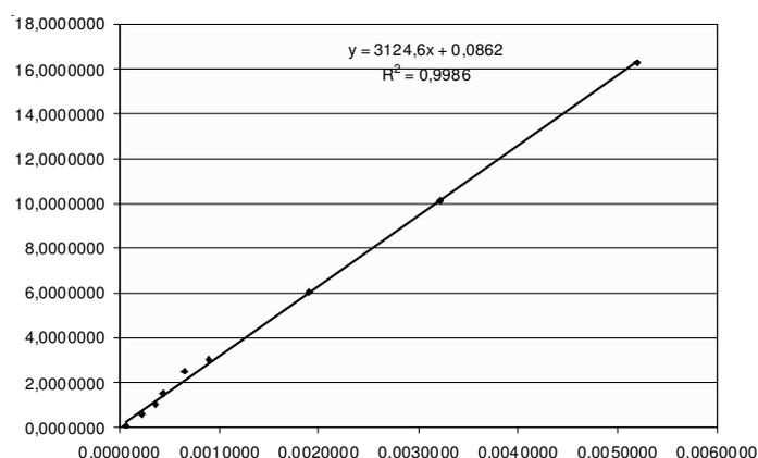
Fig. 1. Calibration curve of the experimental model of tritium storage bed
