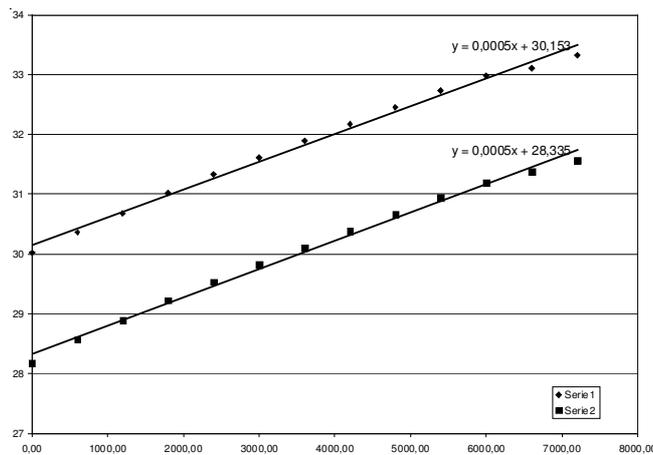
Fig. 7. Temperature *versus* time for P = 2.0 W
