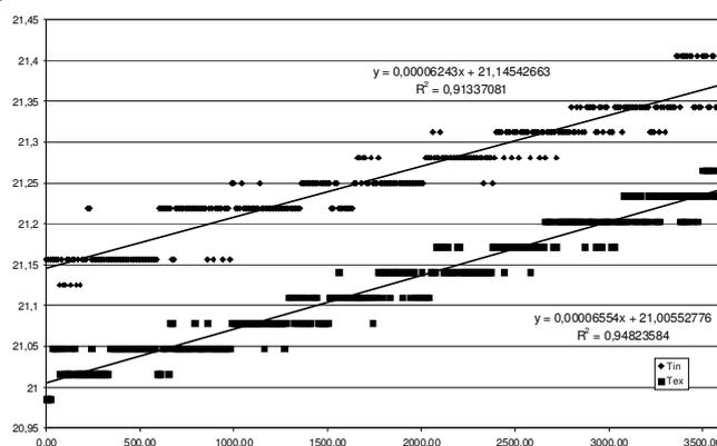
Fig. 3. Temperature *versus* time for  $P = 0.1$  W
