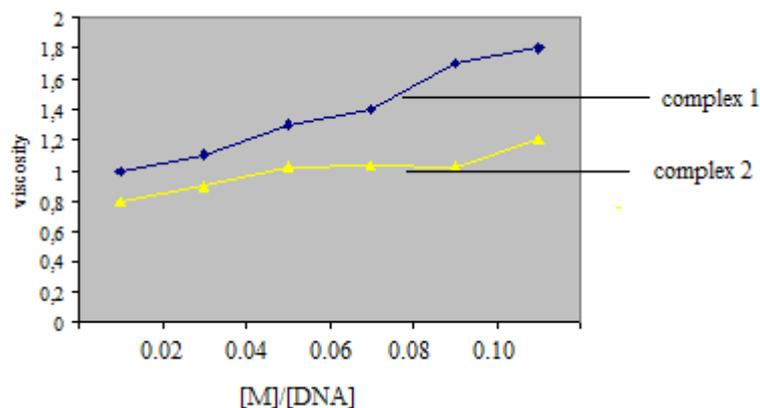
Fig. 7. Effect of increasing amounts of the zinc complexes on the relative viscosity of cat DNA at 30 °C. Where M represents the zinc complexes
