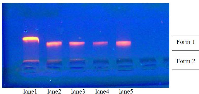
Fig. 4. DNA oxidative cleavage by different concentration of complex **2**. The concentration of  $H_2O_2$  is kept constant at 15 mM and the concentration of the complex is varied. Lane 5 is control DNA in absence of  $H_2O_2$ ; lane 1, lane 2, lane 3 and lane 4 are DNA + [complex **2**]. Each of lanes shows the cleavage experiment in presence of  $H_2O_2$ , respectively
