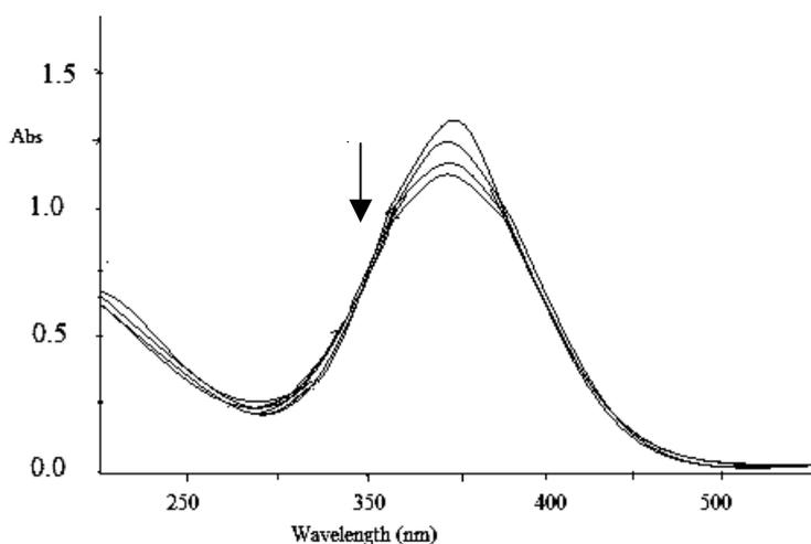
Fig. 5. Absorption spectra of complex **1** in the presence of increasing amounts of cat DNA. Arrow shows the intensities changes upon increasing DNA concentration
