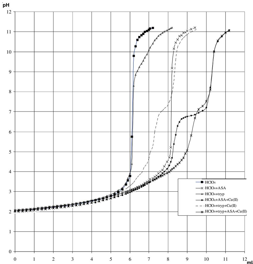
Fig. 1. Potentiometric titration curves of  $\text{HClO}_4$ ,  $\text{HClO}_4 + \text{ASA}$ ,  $\text{HClO}_4 + \text{Tryp}$ ,  $\text{HClO}_4 + \text{Cu(II)}$  +  $\text{Tryp}$ ,  $\text{HClO}_4 + \text{Cu(II)} + \text{ASA}$  and  $\text{HClO}_4 + \text{Cu(II)} + \text{ASA} + \text{Tryp}$  ( $I = 0.11$ ;  $T = 25 (\pm 1) ^\circ\text{C}$ )
