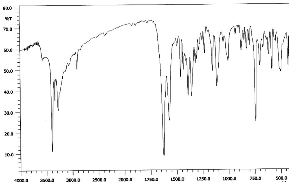
Fig. 5. IR spectrum of Cu(II)-Tryp (1:1) complex, precipitated at pH = 7.20
