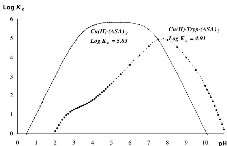
Fig. 2. Conditional formation curves of Cu(II)-Tryp-(ASA)<sub>2</sub> and Cu(II)-(ASA)<sub>2</sub> complexes (I = 0.11; T = 25 (± 1) °C) and the binding constants of aspirin (ASA) to Cu(II) and Cu(II)-Tryp complex
