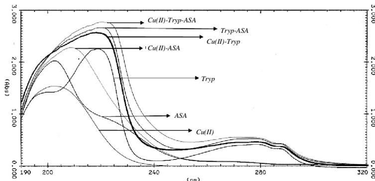
Fig. 4. Spectra pertaining to the comparative investigation of formation of Cu(II)-Tryp-ASA (1:1:2) complex (pH = 5.50). The interaction was best observed at 210 nm, at 25 °C. Conc: Cu(II) =  $8.00 \times 10^{-5}$  M ; Tryp =  $8.00 \times 10^{-5}$  M; ASA =  $1.60 \times 10^{-4}$  M
