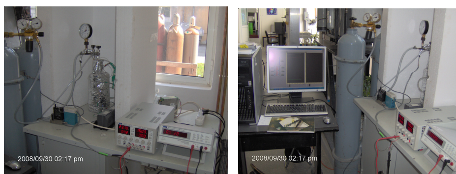
Fig. 1. Experimental setup for the calibration of the tritium storage bed
