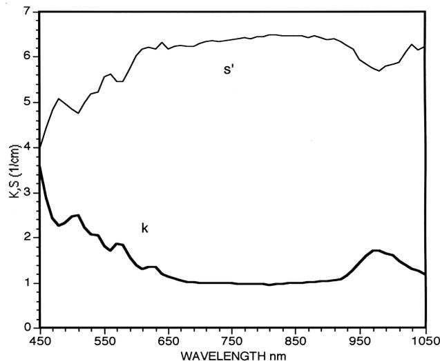
Fig. 3. Absorption and scattering spectrum of Hails potato incubated in photofrin II
