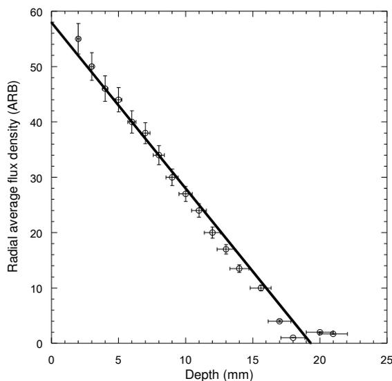
Fig. 1. Attenuation of radial flux in potato tissue
