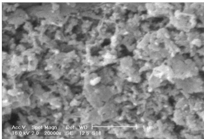
Fig. 4. Scanning electron micrograph of polyaniline in aqueous/non-aqueous (water/ethyl acetate) media. Reaction conditions: (ammonium persulphate = 10 g/L, aniline monomer  $10.75 \times 10^{-2}$  mol/L, sodium dodecylbenzenesulfonate = 9 g/L, volume of solution 100 mL (75/25 % v/v), reaction time 4 h at room temperature)
