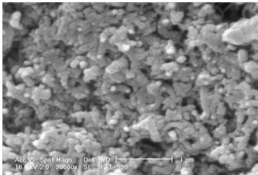
Fig. 6. Scanning electron micrograph of polyaniline in polyaniline aqueous/non-aqueous (water/ethyl acetate) media. Reaction conditions: (ammonium persulphate = 10 g/L, aniline monomer  $10.75 \times 10^{-2}$  mol/L, hydroxypropylcellulose = 9g/L, volume of solution 100 mL (75/25 % v/v), reaction time 4 h at room temperature)
