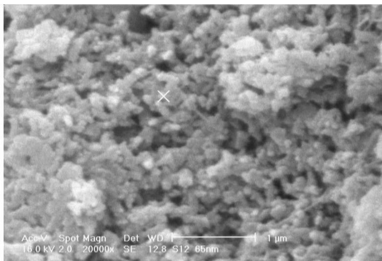
Fig. 2. Scanning electron micrograph of polyaniline in aqueous/non-aqueous (water/ethyl acetate) media. Reaction conditions: (ammonium persulphate = 10 g/L, aniline monomer  $10.75 \times 10^{-2}$  mol/L, sodium dodecylbenzenesulfonate = 3 g/L, volume of solution 100 mL (75/25 % v/v), reaction time 4 h at room temperature)
