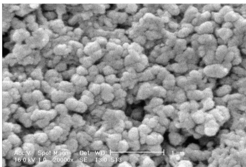
Fig. 3. Scanning electron micrograph of polyaniline in aqueous/non-aqueous (water/ethyl acetate) media. Reaction conditions: (ammonium persulphate = 10 g/L, aniline monomer  $10.75 \times 10^{-2}$  mol/L, poly(vinyl alcohol) = 3 g/L, volume of solution 100 mL (75/25 % v/v), reaction time 4 h at room temperature)
