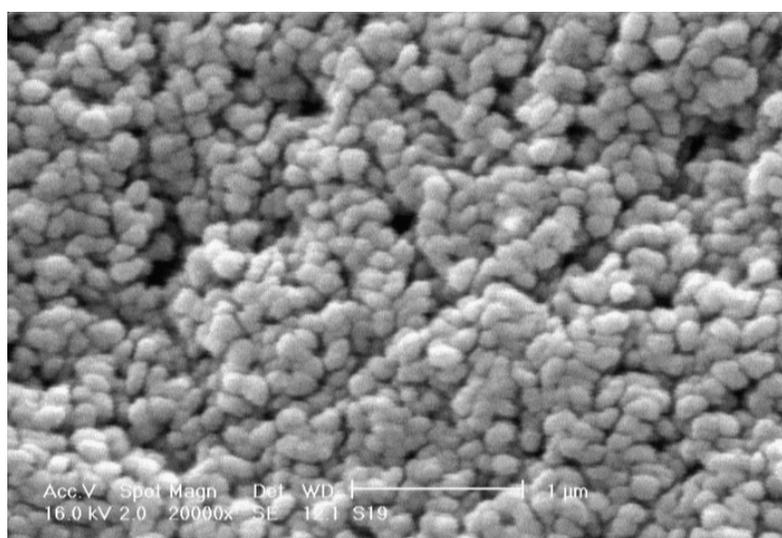
Fig. 5. Scanning electron micrograph of polyaniline in aqueous/non-aqueous (water/ethyl acetate) media. Reaction conditions: (ammonium persulphate = 10 g/L, aniline monomer  $10.75 \times 10^{-2}$  mol/L, poly(vinyl alcohol) = 9 g/L, volume of solution 100 mL (75/25 % v/v), reaction time 4 h at room temperature)
