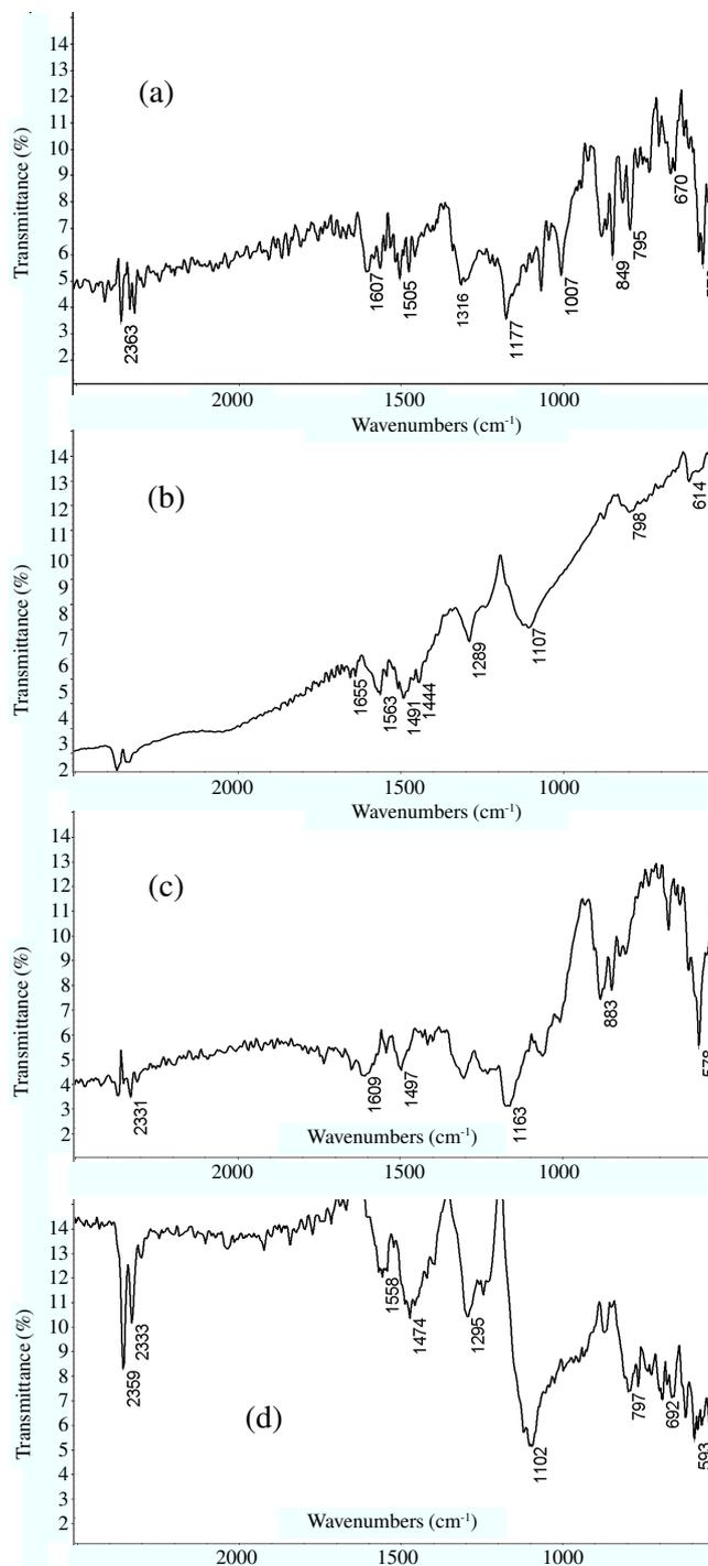
Fig. 7. FTIR spectra of (a) pure polyaniline without surfactant and with (b) DBSNa, (c) PVA and (d) HPC were used as surfactant
