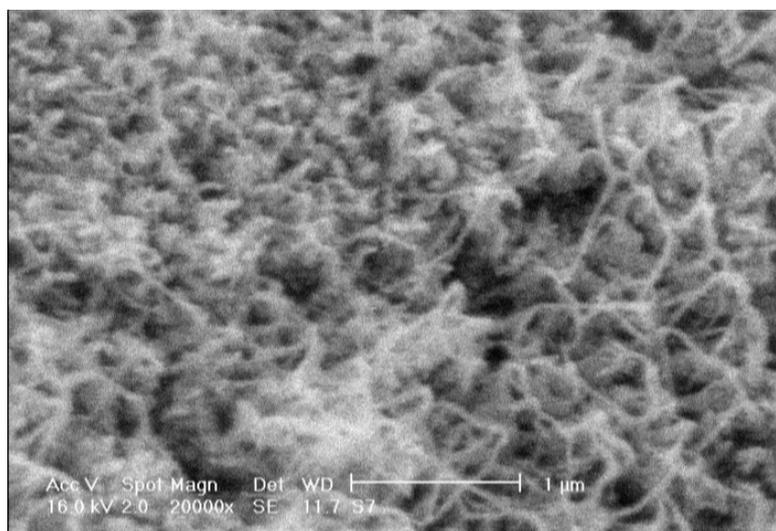
Fig. 1. Scanning electron micrograph of polyaniline in aqueous/non-aqueous (water/ethyl acetate) media. Reaction conditions: (ammonium persulphate = 10 g/L, aniline monomer  $10.75 \times 10^{-2}$  mol/L, volume of solution 100 mL (75/25 % v/v), reaction time 4 h at room temperature)
