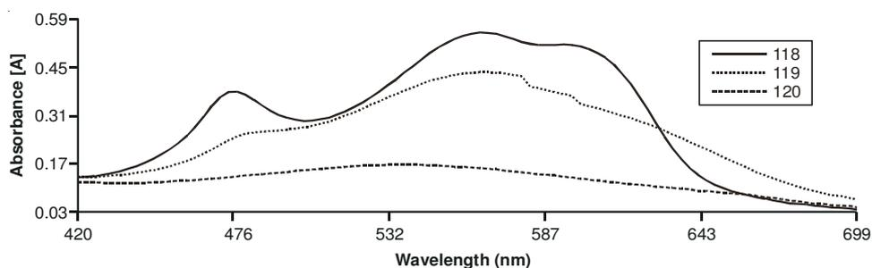
Fig.1. Absorption spectrum for the formaldehyde-cresyl violet- $\text{BrO}_3^-$ -system with time. Conditions:  $\text{H}_2\text{SO}_4$ , 1 M; cresyl violet,  $1.87 \times 10^{-4}$  M;  $\text{BrO}_3^-$   $2.7 \times 10^{-3}$  M; formaldehyde 0.4  $\mu\text{g/mL}$ , temperature, 27  $^\circ\text{C}$ ; interval time for each scan, 0.5, 1.5, 2.5 and 3.5 from initiation of the reaction
