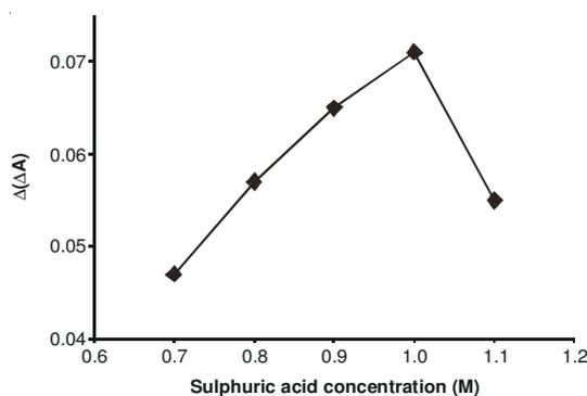
Fig. 2. Effect of  $H_2SO_4$  concentration on the analytical signal, conditions: cresyl violet,  $1.2 \times 10^{-4}$  M;  $BrO_3^-$   $3.0 \times 10^{-3}$  M; formaldehyde  $0.4 \mu\text{g/mL}$ , temperature,  $27^\circ\text{C}$  and time of 1.5 min from initiation of the reaction
