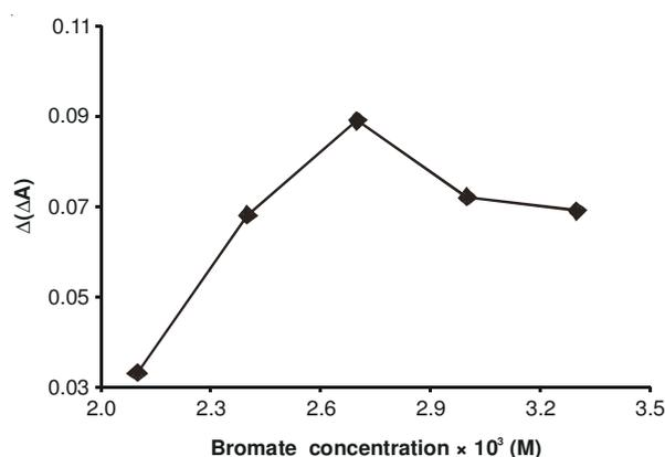
Fig. 4. Influence of  $\text{BrO}_3^-$  concentration on the analytical signal, conditions:  $\text{H}_2\text{SO}_4$ , 1 M; cresyl violet  $1.87 \times 10^{-4}$  M formaldehyde  $0.4 \mu\text{g/mL}$ ; temperature,  $27^\circ\text{C}$  and time of 1.5 min from initiation of the reaction
