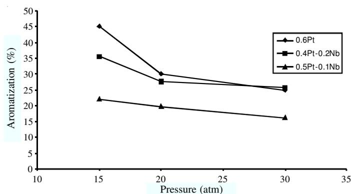
Fig. 5. Effect of pressure on selectivity aromatization % (temperature = 480 °C)
