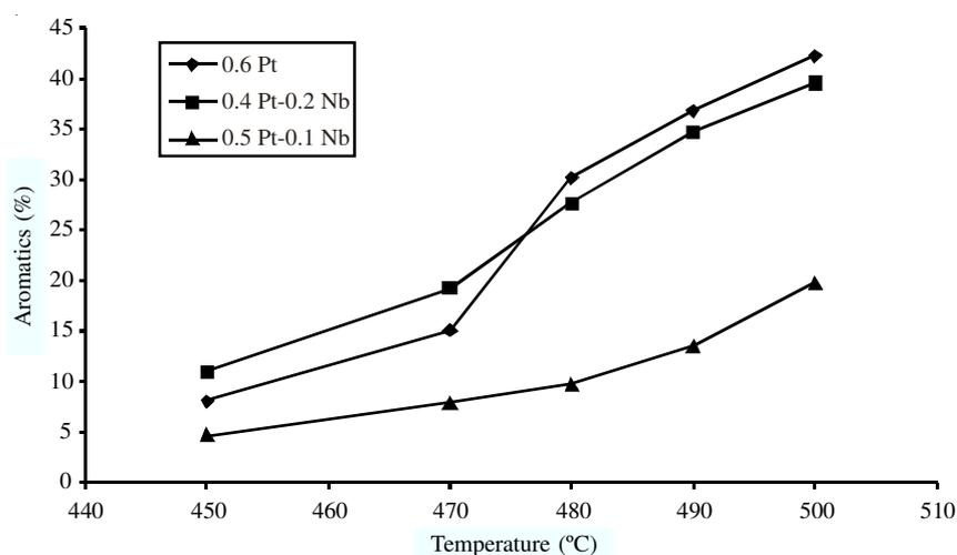
Fig. 3. Effect of temperature on selectivity aromatization % (pressure = 20 atm)
