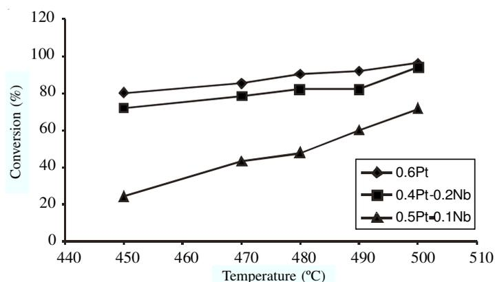
Fig. 1. Effect of temperature on conversion % (pressure = 20 atm)
