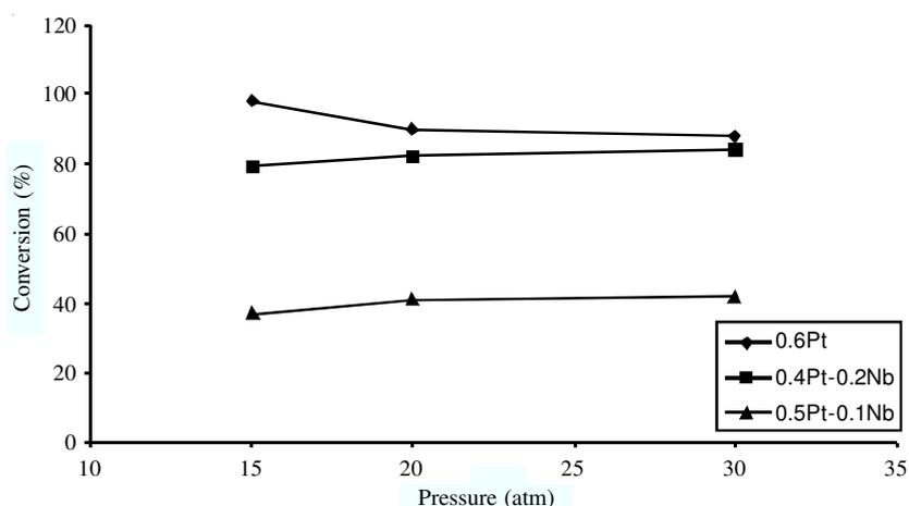
Fig. 4. Effect of pressure on conversion % (temperature = 480 °C)
