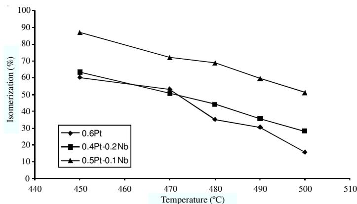
Fig. 2. Effect of temperature on selectivity isomerization % (pressure = 20 atm)
