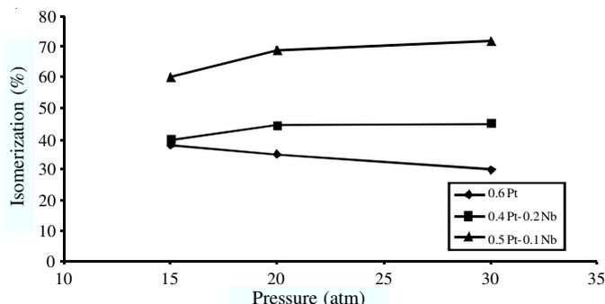
Fig. 6. Effect of pressure on selectivity isomerization % (temperature = 480 °C)
