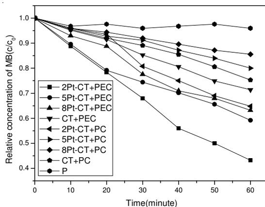
Fig. 5. Dependence of relative concentration ( $c/c_0$ ) of methylene blue in the aqueous solution with different Pt-CNT/TiO<sub>2</sub> electrodes on time of PEC, PC and P reaction. (PEC: Visible light irradiation using the electrodes with a potential of 6 V; PC: Visible light irradiation using the electrodes; P: Only visible light irradiation)
