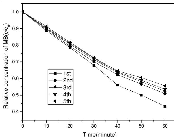
Fig. 6. Effect of reuse of 2Pt-CT electrode on the degradation of methylene blue in the aqueous solution with photoelectrocatalytic reaction. (PEC: Visible light irradiation using the electrodes with a potential of 6 V)
