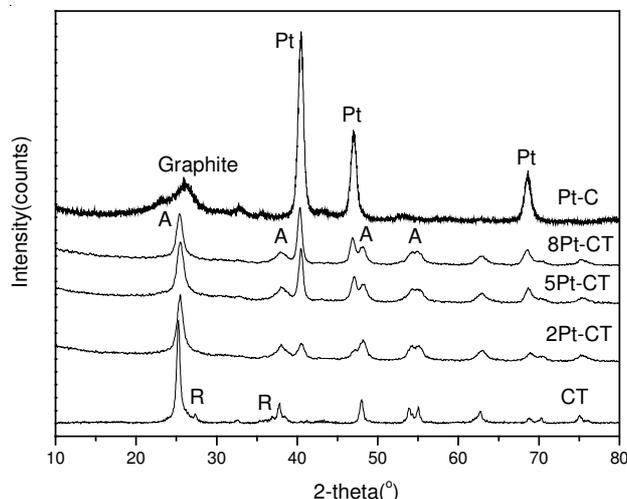
Fig. 1. XRD patterns of CNT/TiO<sub>2</sub>, Pt-CNT and Pt-CNT/TiO<sub>2</sub> composites
