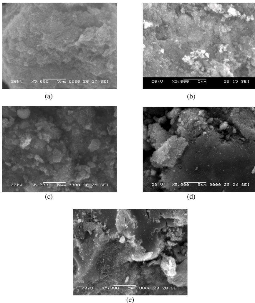
Fig. 2. SEM images obtained from powdered CNT/TiO<sub>2</sub>, Pt-CNT and Pt-CNT/TiO<sub>2</sub> composites; (a) Pt-C, (b) CT, (c) 2Pt-CT, (d) 5Pt-CT and (e) 8Pt-CT
