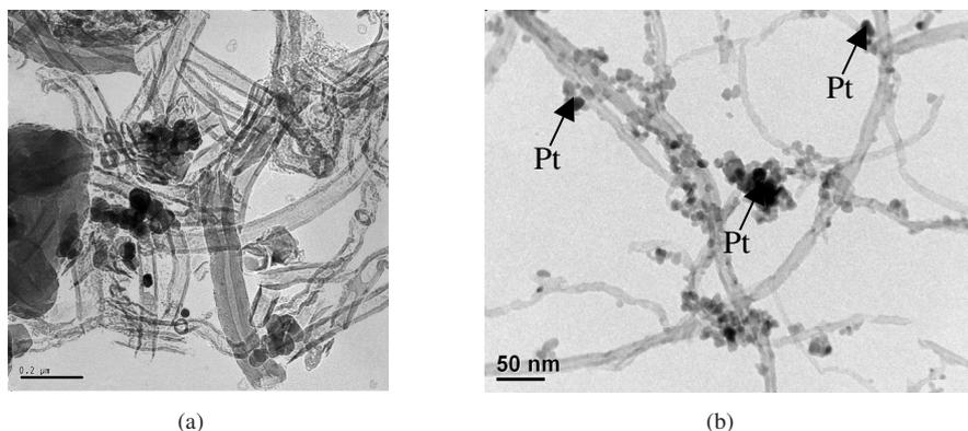
Fig. 3. TEM micrographs obtained from powdered CNT/TiO<sub>2</sub> and Pt-CNT/TiO<sub>2</sub> composites; (a) CT, (b) 5Pt-CT
