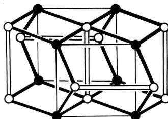
Fig. 1. Structural model of the pn- $T_d$ -type host,  $M(pn)M'(CN)_4$ , open circle, 6-coordinate M; solid circle, tetragonal M'; open column, a pn ligand; thick line, CN bridge and thin line, edge of cavity
