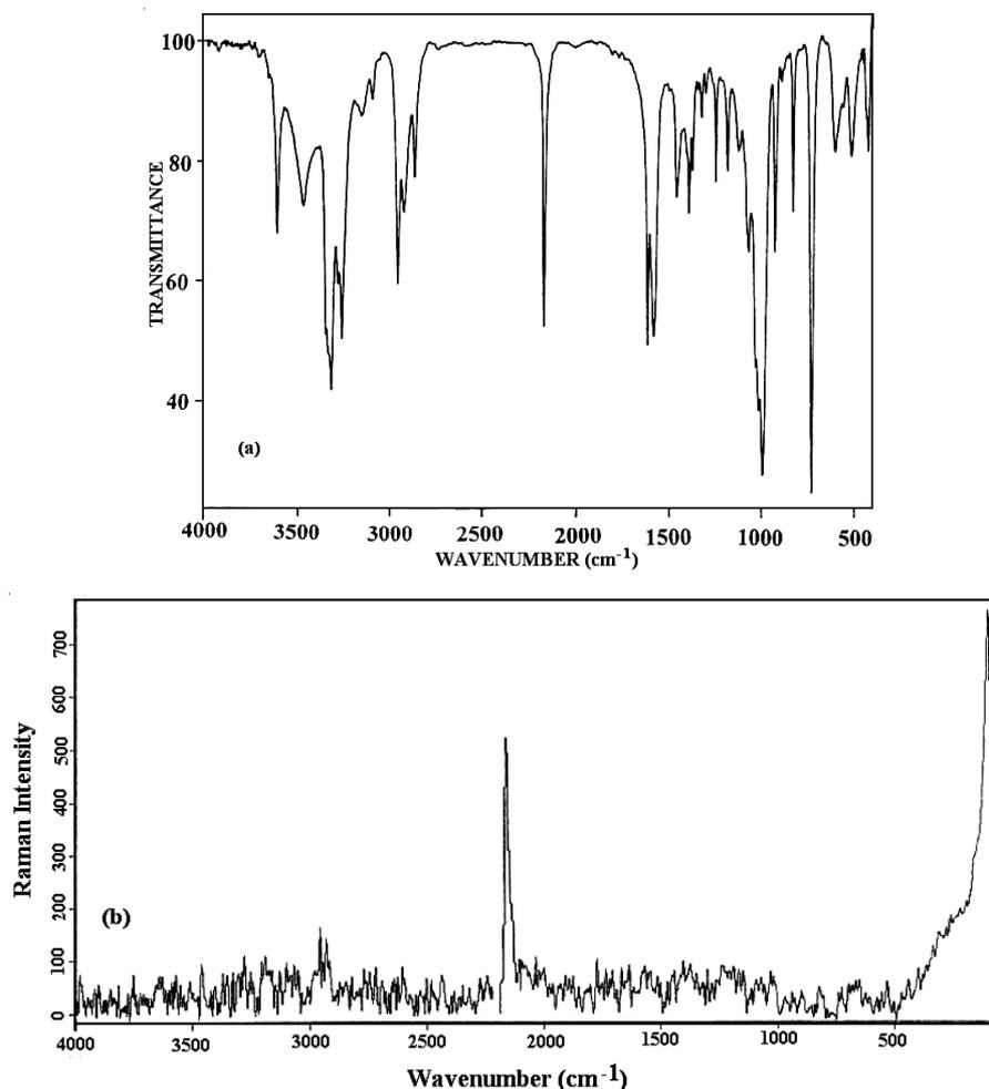
Fig. 2. The FT-IR (in KBr) (a) and FT-Raman (b) spectrum of the Cd-pn-Hg-Thi clathrate
